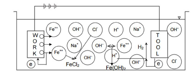
Fe => Fe<sup>+2</sup> +2e<sup>-1</sup> Anode: Cathode:  $H_2O => H^+ + OH^-$ NaCl => Na<sup>+</sup> + Cl<sup>-</sup> **Electrolyte:**  $Fe^{+2} + 4Cl^{-} => 2FeCl_{2}$  $Fe^{+2} + 4OH^{-} => 2Fe(OH)_{2}$ Na<sup>+</sup>+OH<sup>-</sup> => NaOH Dr. Vikas Gupta, CDLSIET, Panniwala
