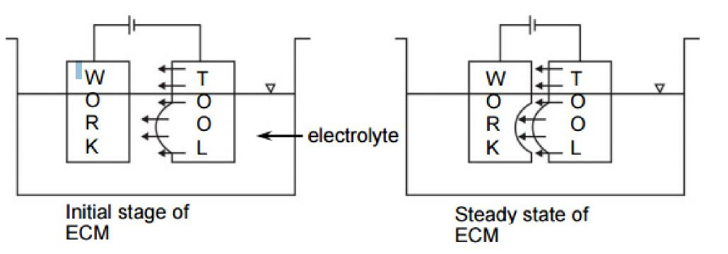
Fig. 1 Schematic principle of Electro Chemical Machining (ECM)
