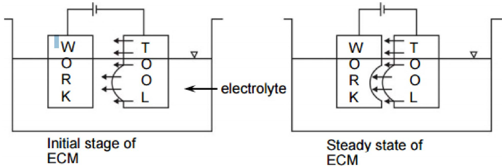
**Fig. 1** Schematic principle of Electro Chemical Machining (ECM)
