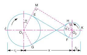
Fig. 11.12. Length of a cross belt drive.
