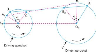
Fig. 11.27. Kinematic of chain drive.
