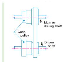
Fig. 11.8. Stepped or cone pulley drive.
