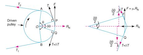
Fig. 11.15. Ratio of driving tensions for flat belt.
