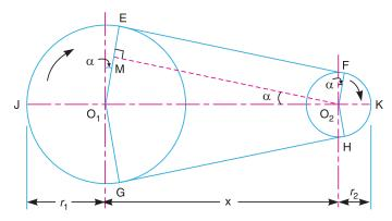
Fig. 11.11. Length of an open belt drive.
