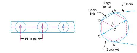
Fig. 11.24. Pitch of the chain. Fig. 11.25. Pitch circle diameter of the chain sprocket.
