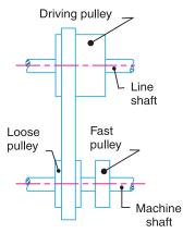
Fig. 11.9. Fast and loose pulley drive.
