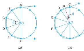
Fig. 11.26. Relation between chain speed and angular velocity of sprocket.
