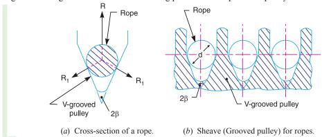
Fig. 11.22. Rope and sheave.
