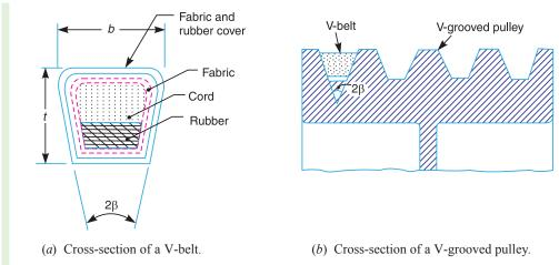
Fig. 11.19. V-belt and V-grooved pulley.
