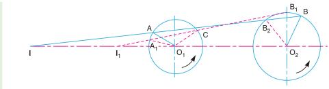
Fig. 11.28. Angular velocities of the two sprockets.
