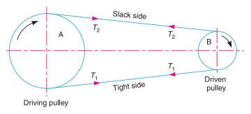
Fig. 11.14. Power transmitted by a belt.
