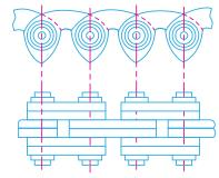
Fig. 11.33. Inverted tooth or silent chain.
