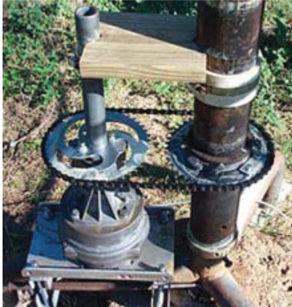
The chains are mostly used to transmit motion and power from one shaft to another, when the distance between the centres of the shafts is short such as in bicycles, motor cycles, agricultural machinery, road rollers, etc.
