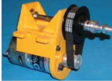
$$\text{or } \frac{N_4}{N_1} = \frac{d_1 \times d_3}{d_2 \times d_4} \quad \dots (\because N_2 = N_3, \text{ being keyed to the same shaft})$$
