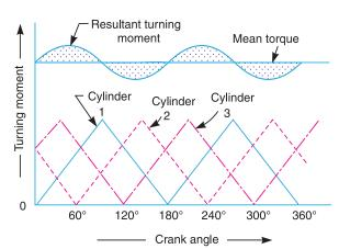
Fig. 16.3. Turning moment diagram for a multi-cylinder engine.
