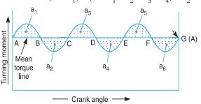
Fig. 16.4. Determination of maximum fluctuation of energy.
