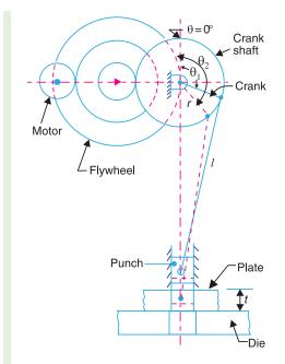
**Fig. 16.22.** Operation of flywheel in a punching press.
