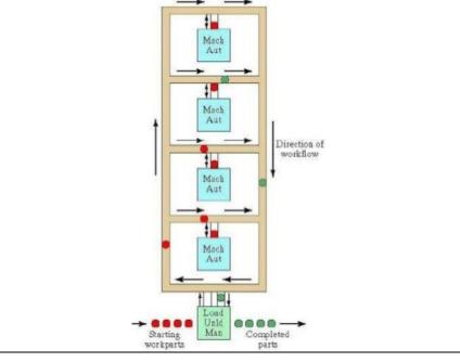
Open Field Type: The configuration of the open field is as shown in the figure. The loading and unloading station is typically located at the same end. The parts will go through all the substations, such as CNC machines, coordinate measuring machines and wash station by thehelp of AGV's from one substation to another.
