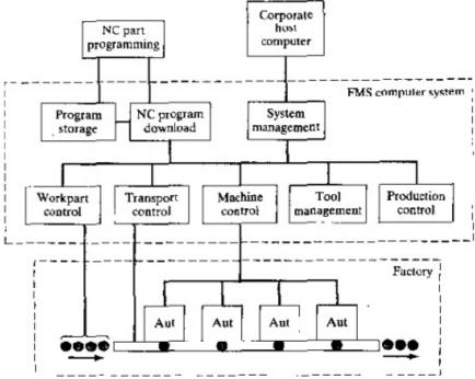
The modular structure of the FMS application software for system control is illustrated in Figure 1.8. It should be noted that an FMS possesses the characteristic architecture or a DNC system. As in other DNC systems. Two-way communication is used. Data and commands an: sent from the central computer to the individual machines and other hardware components, and data on execution and performance are transmitted from the components hack up to the central computer.
