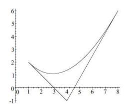
Quadratic Bézier curve with control points  $b_0(1, 2)$ ,  $b_1(4, -1)$ , Suppose four control points  $b_0$ ,  $b_1$ ,  $b_2$ , and  $b_3$  are specified, then the cubic Bézier curve is defined to be
