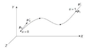
• The parametric equation of a Hermite cubic spline is given by
