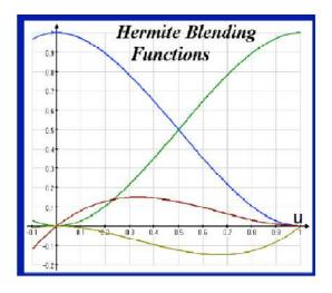
**Example 5**: A parametric cubic curve passes through the points (0,0), (2,4), (4,3), (5,-2) which are parametrized at t = 0,  $\frac{1}{4}$ ,  $\frac{3}{4}$ , and 1, respectively. Determine the geometric coefficient matrix and the slope of the curve when t = 0.5.
