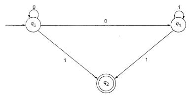
Fig. 3.7 Transition system representing nondeterministic automaton.
