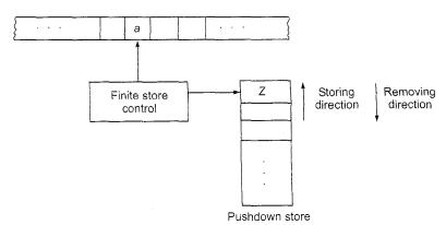
Fig. 7.1 Model of a pushdown automaton.
