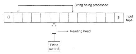
Fig. 3.4 Block diagram of a finite automaton.
