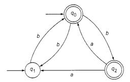
Fig. 5.11 Nondeterministic transition system of Example 5.7.
