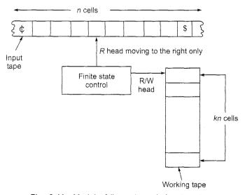
Fig. 9.11 Model of linear bounded automaton.
