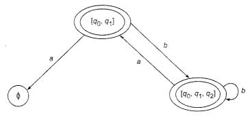
Fig. 5.12 Deterministic transition system for Example 5.7.
