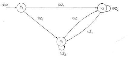
Fig. 3.10 Mealy machine of Example 3.12.
