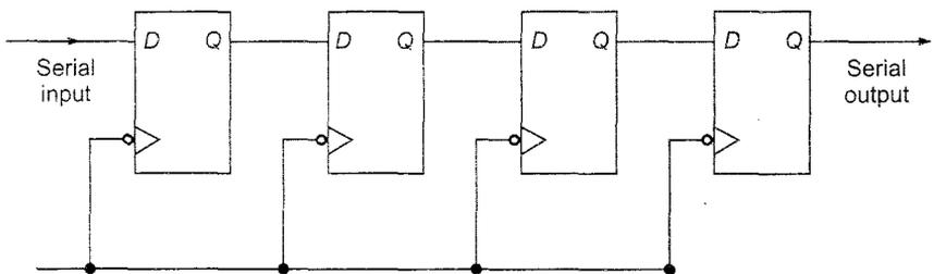
Fig. 3.2 A 4-bit serial shift register using D flip-flops.
