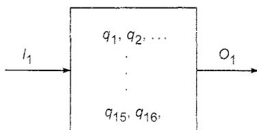
Fig. 3.3 A shift register as a finite-state machine.
