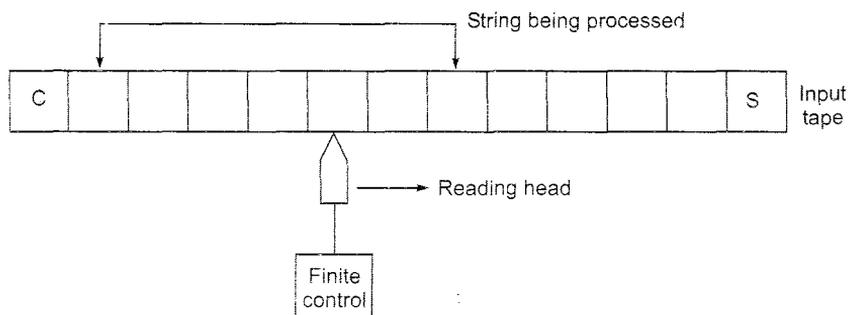
Fig. 3.4 Block diagram of a finite automaton.
