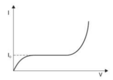
The exponential increase in current is due to ionization of gas by electron collision.
