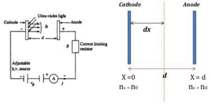
At any distance x from the cathode, let the number of electrons be n<sub>x</sub>.
