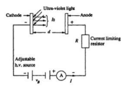
Fig. 2.1 Arrangement for study of a Townsend discharge
