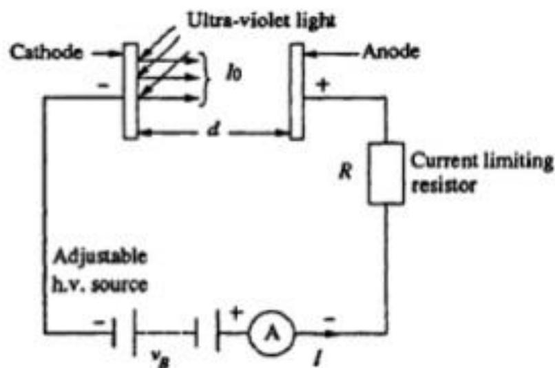
Fig. 2.1 Arrangement for study of a Townsend discharge
