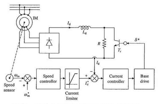
Fig. 6.52 Closed-loop speed control with static rotor resistance control
