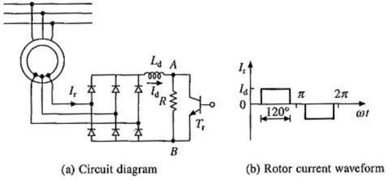
Fig. 6.51 Rotor resistance control employing semiconductor converters
