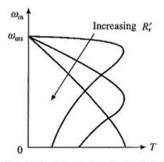
Fig. 6.50 Rotor resistance control
