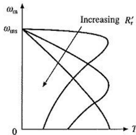
**Fig. 6.50** Rotor resistance control
