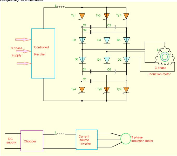
The variable frequency control of an induction motor can also be obtained using CSI. The inductor is connected in series with the input.
