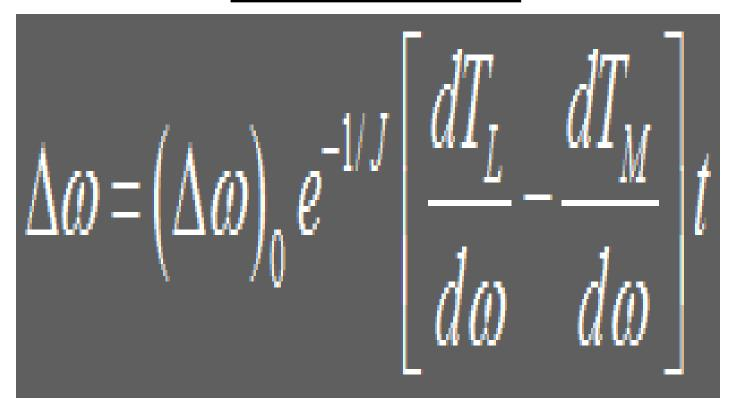
Where,  $(\Delta \omega)$ 0 is the initial value of the deviation in speed. For the stable system the exponent must be negative, so speed increment will disappear with time. The exponent will always be negative if,
