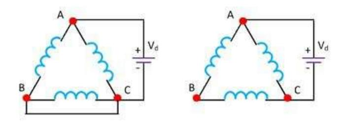
Three Lead Connection of DC Dynamic Braking
