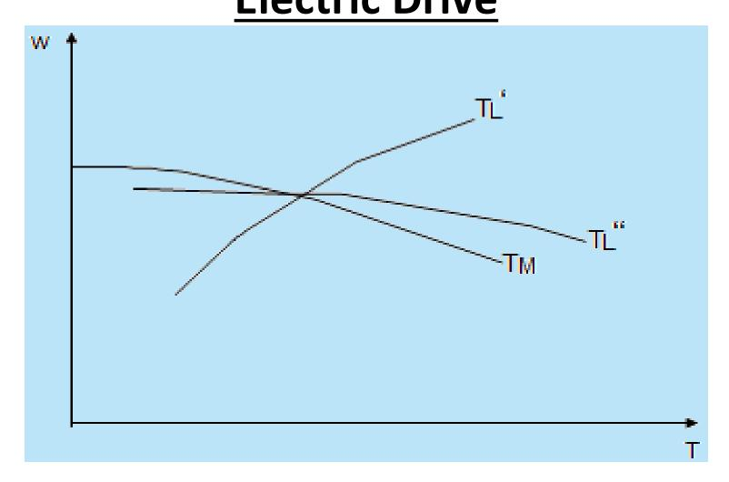
To check the stability at an operating point of the motor, if an increase in speed brings greater
