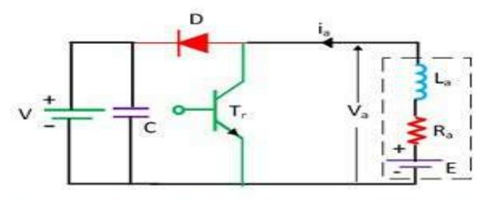
**Regenerative Braking of Separately Excited** Motor by Chopper Control
