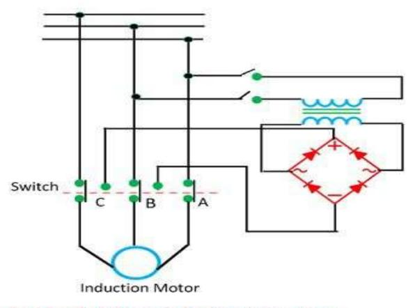
Two Lead DCdynamic Braking Connection Circuit Globe
