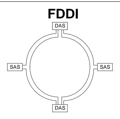
SAS Single Attached Station DAS Dual Attached Station
