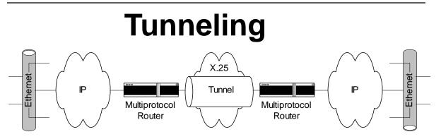
Figure 2.24 Tunneling Using Multiprotocol Routers
