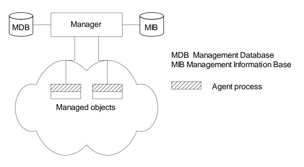
Figure 3.6 Network Configuration with Data and Information Base
