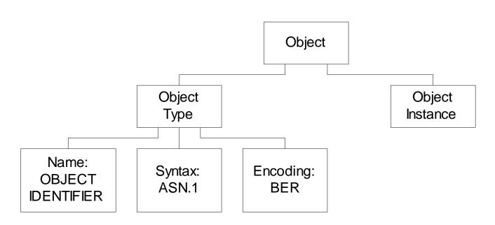
Figure 4.10 Managed Object : Type and Instance
