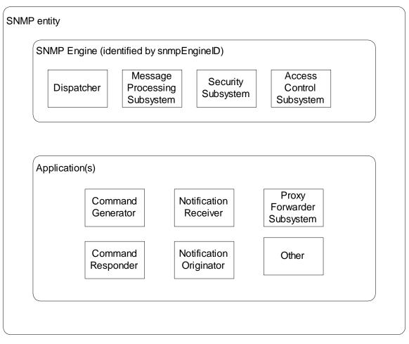
Figure 7.2 SNMPv3 Architecture
