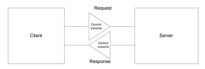
Figure 1.7 Simple Client-Server Model
