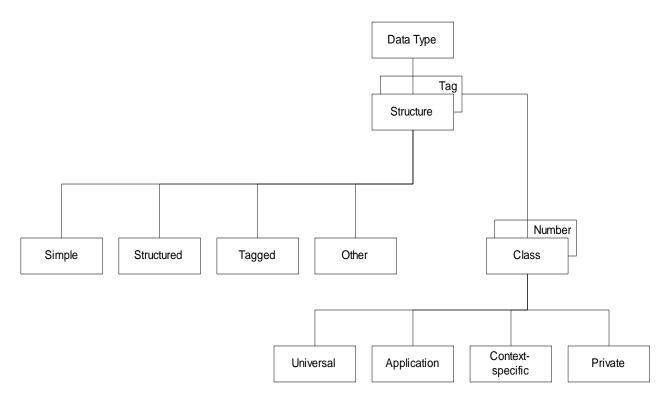
Figure 3.15 ASN.1 Data Type Structure and Tag
