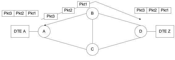
Figure 2.26(b) Virtual Circuit Configuration
