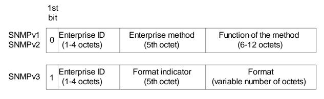
Figure 7.3 SNMP Engine ID
