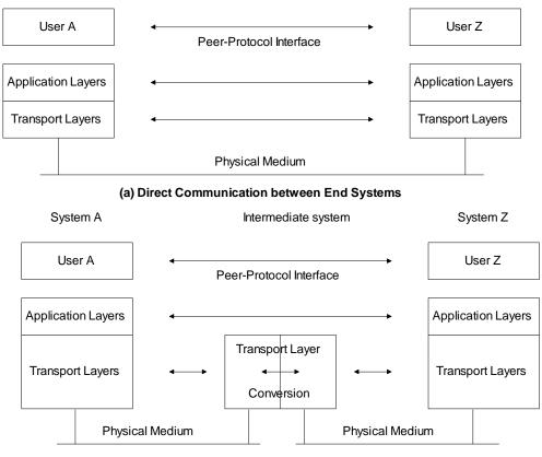
(b) Communication between End Systems via an Intermediate System
