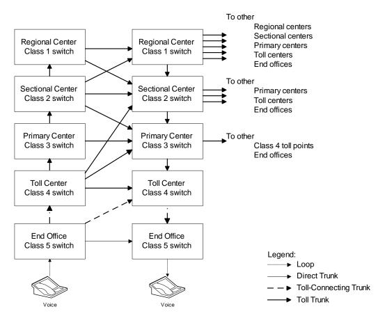
Figure 1.1 Telephone Network Model
