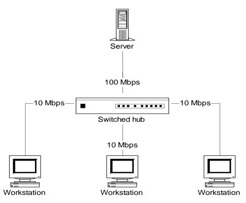
Figure 2.9 Switched Hub in Client-Server Configuration
