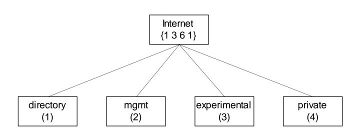
Figure 4.13 Subnodes under Internet Node in SNMPv1
