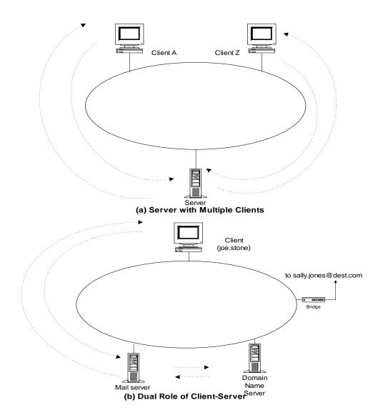
Figure 1.8 Client-Server in Distributed Computing Environment
