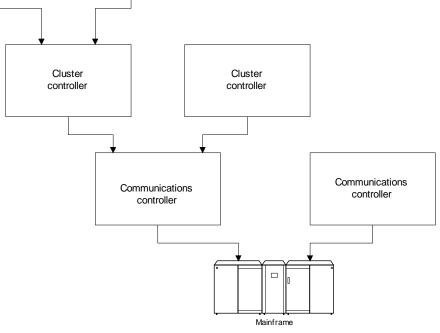
Figure 1.5 IBM Systems Network Architecture Model
