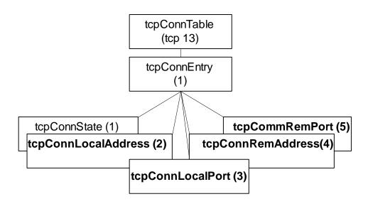
Figure 4.36 TCP Connection Table
