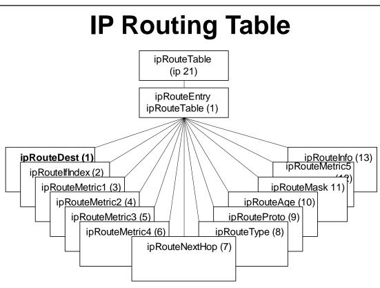
Figure 4.31 IP Routing Table
