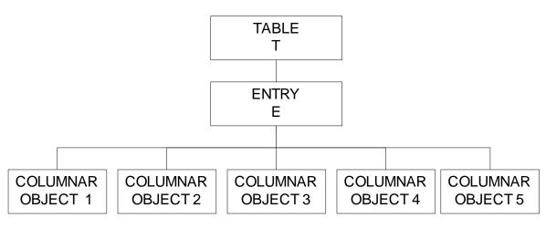
Figure 4.22(a) Multiple Instance Managed Object
