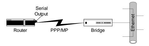
Figure 2.25 Half-Bridge Configuration
