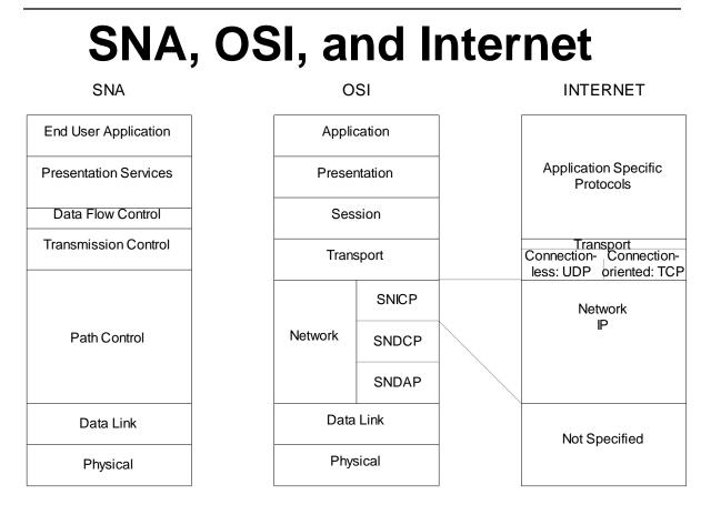
Figure 1.18 Comparison of OSI, Internet, and SNA Protocol Layer Models
