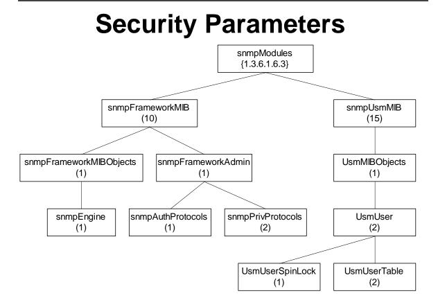
Figure 7.15 SNMPv3 MIB Objects for Security Parameters
