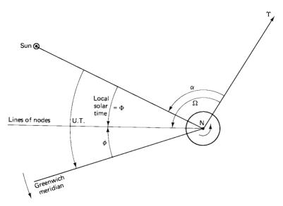
Figure 2.15 The condition for sun synchronicity is that the local solar time should be constant. Local solar time =  $\Omega - \alpha$ , which is also equal to the angle  $\Phi$  shown in Fig. 2.14. This is the local solar time at the ascending node, but a similar situation applies at other latitude crossings.
