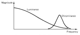
Figure 9.5 Frequency spectra for the luminance and chrominance signals.
