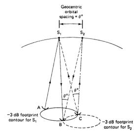
**Figure 13.3** Orbital spacing angle  $\theta$ .
