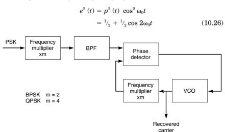
Figure 10.20 Functional block diagram for carrier recovery.
