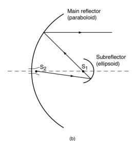
Figure 6.23 Ray paths for (a) Cassegrain and (b) Gregorian antennas.
