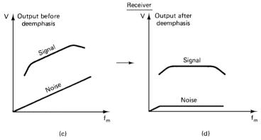
**Figure 9.13** (a) and (b) Effect of preemphasis on the modulating signal frequency response at the transmitter. (c) and (d) Effect of deemphasis on the modulating signal and noise at the receiver output. The deemphasis cancels out the preemphasis for the signal while attenuating the noise at the receiver.
