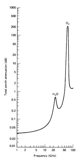
Figure 4.2 Total zenith attenuation at ground level: pressure = 1 atm, temperature = 20°C, and water vapor = 7.5 g/m³. (Adapted from CCIR Report 719-2, with permission from International Telecommunication Union.)
