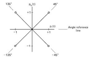
Figure 10.15 Phase diagram for QPSK modulation.
