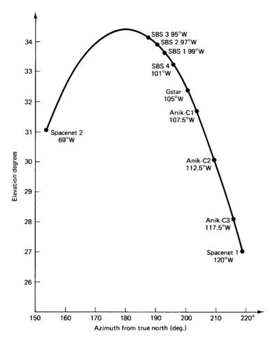
Figure 3.4 Azmuth-elevation angles for an earth station location of  $48.42^\circ N,\,89.26^\circ W$  (Thunder Bay, Ontario). Ku-band satellites are shown.
