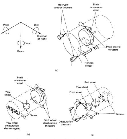
Figure 7.8 Alternative momentum wheel stabilization systems: (a) one-wheel; (b) two-wheel; (c) three-wheel. (Reprinted with permission from Spacecraft Attitude Determination and Control, edited by James R. Wertz. Copyright @ 1984 by D. Reidel Publishing Company, Dordrecht, Holland.)
