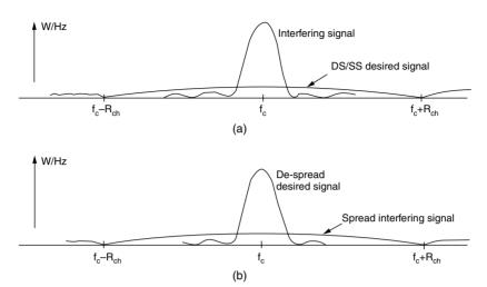
**Figure 14.39** (a) Spectrum of an interfering, nonspread signal along with the spread desired signal; (b) the effect of the de-spreading operation on the desired signal resulting in spread of the interfer.
