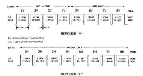
Figure 7.31 Anik-E1 frequency and polarization plan, Ku-band. (Courtesy of Telesat Canada.)
