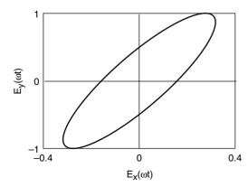
Figure 5.4 Elliptical polarization.
