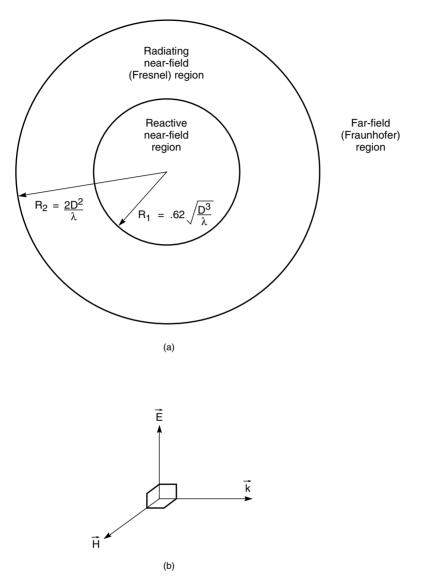
Figure 6.4  $\,$  (a) The electromagnetic field regions surrounding an antenna. (b) Vector diagrams in the far-field region.
