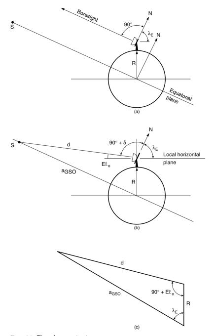
Figure 3.5 The polar mount antenna.
