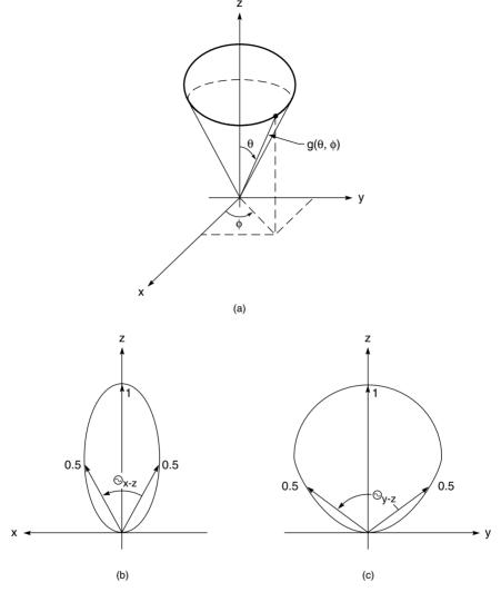
Figure 6.6 (a) A radiation pattern. (b) The beamwidth in the H-plane. (c) The beamwidth in the E-plane.
