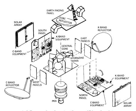
Figure 7.26 Anik-E spacecraft configuration. (Courtesy of Telesat Canada.)
