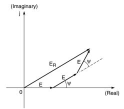
**Figure 6.27** Phasor diagram for the in-line array of dipoles.
