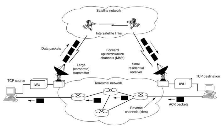
Figure 15.9 Asymmetric reverse ACK channel configuration. (From Ghani and Dixit, 1999. © 1999 IEEE.)
