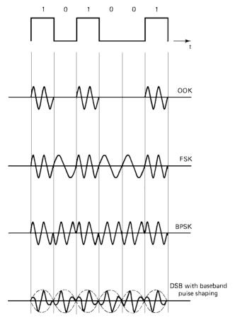
Figure 10.11 Some binary digital modulation formats.
