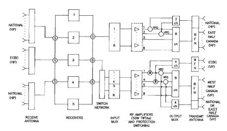
Figure 7.30 Ku-band transponder functional diagram for Anik-E. (Courtesy of Telesat Canada.)
