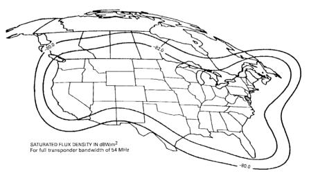
Figure 7.33 Anik-E ECBC saturated flux density (SFD) contours, Ku-band horizontal polarization (HP) (prelaunch predicts, preliminary). (Courtesy of Telesat Canada.)
