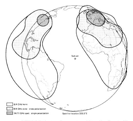
Figure 7.23 INTELSAT V Atlantic satellite transmit capabilities. (*Note:* The 14/11-GHz spot beams are steerable and may be moved to meet traffic requirements as they develop.) (*From Intelsat Document BG-28-72E M/6/77, with permission.*)
