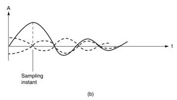
**Figure 10.9** (a) Pulse ringing. (b) Sampling to avoid ISI.
