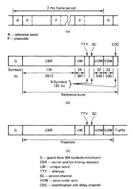
Figure 14.14 (a) Intelsat 2-ms frame; (b) composition of the reference burst R; (c) composition of the preamble P. (QPSK modulation is used, giving 2 bits per symbol. Approximate time intervals are shown.)
