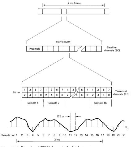
$\textbf{Figure 14.20} \quad \text{Preassigned TDMA frame in the Intelsat system}.$
