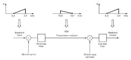
Figure 9.2 A basic SSB transmission scheme.
