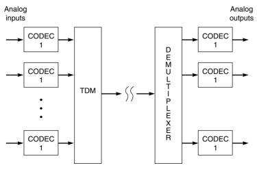
Figure 10.6 A basic TDM system.
