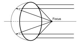
**Figure 6.16** The focusing property of a paraboloidal reflector.
