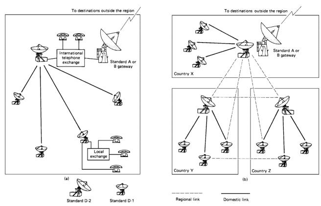
Figure 1.4 (a) Typical Vista application; (b) domestic/regional Vista network with standard A or B gateway. (From Colino, 1985; courtesy of ITU Telecommunication Journal.)
