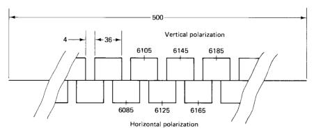
$\textbf{Figure 7.12} \quad \text{Section of an uplink frequency and polarization plan. Numbers refer to frequency in megahertz. } \\$
