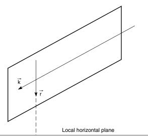
**Figure 5.8** The reference plane for the direction of propagation and the local gravity direction.
