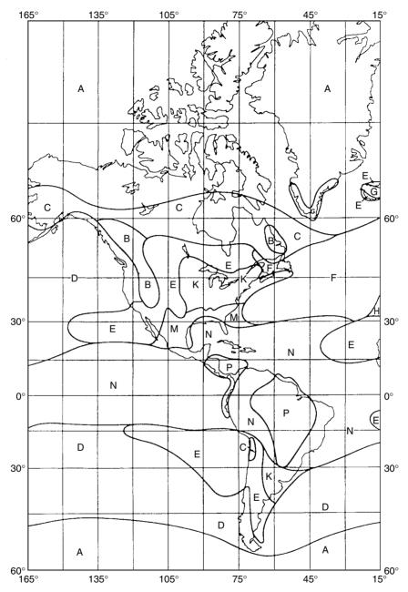
Figure 16.8 Rain climatic zones. Refer to Table 16.2. (From Rec. ITU-R PN.837-1, with permission from the copyright holder ITU. Sole responsibility for the reproduction rests with the author. The complete volume of the ITU material from which the material is extracted can be obtained from the International Telecommunication Union, Sales and Marketing Service, Place des Nations-CH-1211, Geneva 20, Switzerland.)
