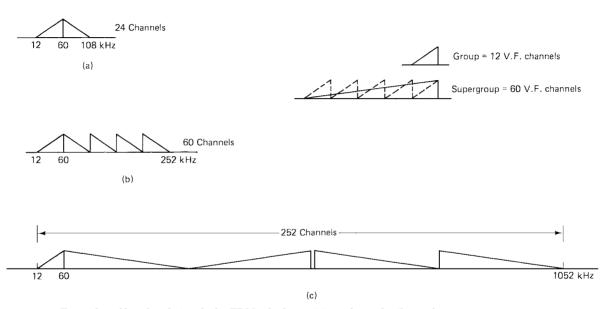
Figure 9.4 Examples of baseband signals for FDM telephony: (a) 24 channels; (b) 60 channels; (c) 252 channels.
