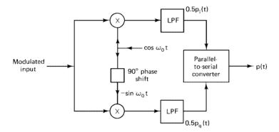
Figure 10.16 Demodulator circuit for QPSK modulation.
