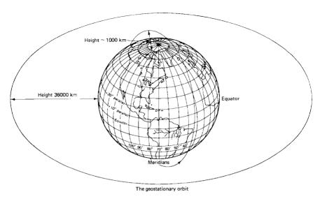
Figure 1.6 Geostationary orbit and one possible polar orbit.
