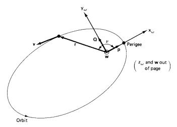
Figure 2.8 Perifocal coordinate system (PQW frame).
