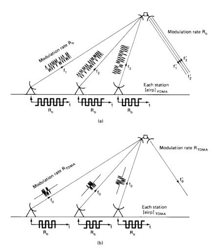
Figure 14.24 (a) FDMA network; (b) TDMA network.
