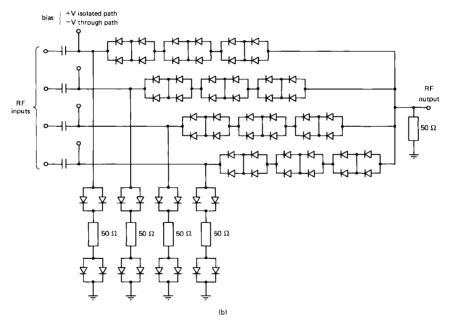
Figure 14.31 (a) 4  $\times$  4 switch matrix; (b) circuit diagram of redundant SP4T switch element. (From Watt, 1986; reprinted with permission of IEEE, London.)
