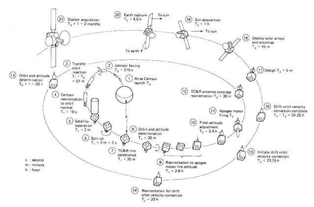
Figure 3.11 From launch to station of INTELSAT V (by Atlas-Centaur). (© KDD Engineering & Consulting, Inc., Tokyo. From Satellite Communications Technology, edited by K. Miya, 1981.)
