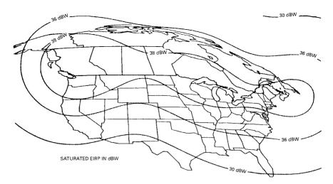
$\begin{tabular}{ll} Figure 7.28 & Anik-E typical C-band coverage, saturated EIRP in dBW (prelaunch EIRP predicts-preliminary). (Courtesy of Telesat Canada.) \end{tabular}$
