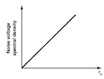
Figure 9.11 Noise voltage spectral density for FM.
