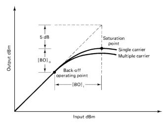
**Figure 12.7** Input and output back-off relationship for the satellite traveling-wave-tube amplifier;  $[BO]_i = [BO]_0 + 5 \text{ dB}$ .
