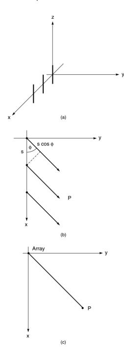
Figure 6.26 An in-line array of dipoles.
