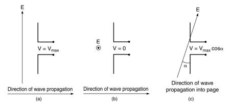
Figure 5.5 Linear polarization relative to a receiving dipole.
