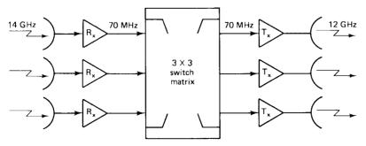
Figure 14.28 Switch matrix in the R.F. link.
