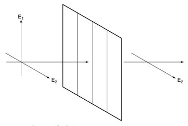
Figure 5.6 A wire grid polarizer.
