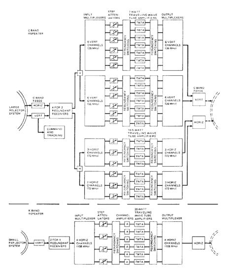
Figure 7.24 Communications subsystem functional diagram for Morelos. (Courtesy of Hughes Aircraft Company Space and Communications Group.)
