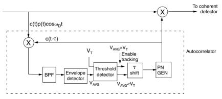
Figure 14.36 Acquisition of a carrier in a CDMA system.
