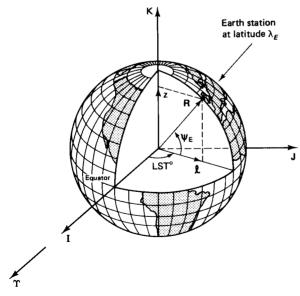
Figure 2.10 Position vector  ${\bf R}$  of the earth relative to the  ${\bf IJK}$  frame.
