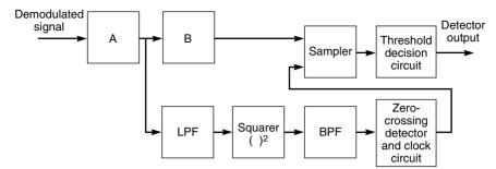
Figure 10.21 Functional block diagram for bit-timing recovery.
