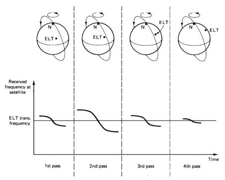
Figure 1.9 Showing the Doppler shift in received frequency on successive passes of the satellite. ELT= emergency locator transmitter.
