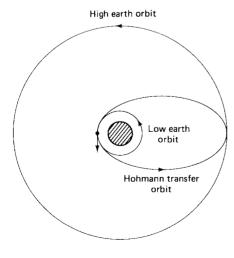
Figure 3.10 Hohmann transfer orbit.
