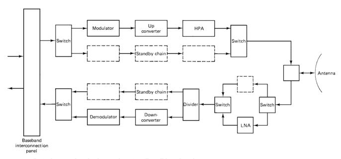
$\begin{array}{ll} \textbf{Figure 8.5} & \text{Basic elements of a redundant earth station.} \ (\textit{From Telesat Canada}, 1983; \textit{courtesy} \\ \textit{of Telesat Canada}.) \end{array}$
