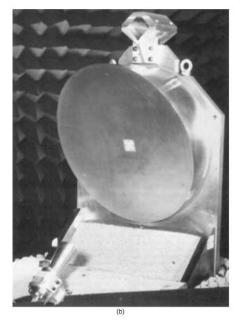
Figure 6.21  $\ (a)$  Ray paths for an offset reflector.  $\ (b)$  The offset feed for a paraboloidal reflector.  $\ (From\ Brain\ and\ Rudge,\ 1984,\ with\ permission.)$
