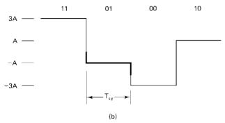
**Figure 10.3** Encoding of 11010010 in (a) binary polar NRZ and (b) quarternary polar NRZ.
