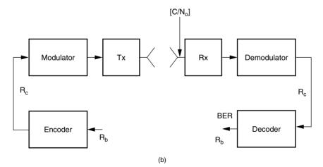
Figure 11.7 Comparing links with and without FEC.
