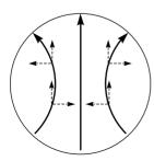
**Figure 6.11** Aperture field in a smooth-walled conical horn.
