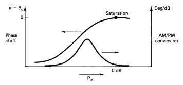
Figure 7.19 Phase characteristics for a TWT.  $\theta$  is the input-to-output phase shift, and  $\theta_S$  is the value at saturation. The AM/PM curve is derived from the slope of the phase shift curve.
