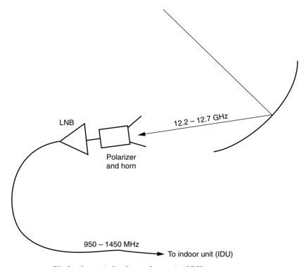
Figure 16.5 Block schematic for the outdoor unit (ODU).
