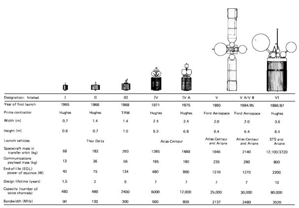
Figure 1.1 Evolution of INTELSAT satellites. (From Colino 1985; courtesy of ITU Telecommunications Journal.)
