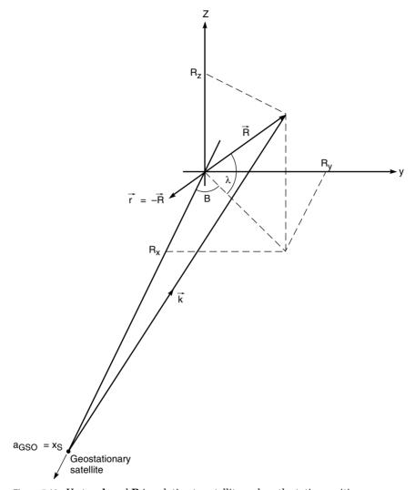
Figure 5.10 Vectors  ${\bf k}$  and  ${\bf R}$  in relation to satellite and earth station positions.
