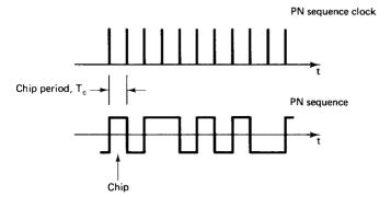
Figure 14.32 PN binar sequence. One element is known as a chip.
