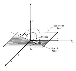
Figure 2.9 Geocentric-equatorial coordinate system (IJK frame).
