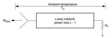
Figure 12.5 Network matched at both ends, to a terminating resistor  ${\cal R}_T$  at one end and an antenna at the other.
