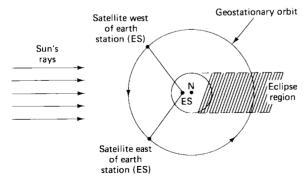
Figure 3.9 A satellite east of the earth station enters eclipse during daylight (busy) hours at the earth station. A satellite west of the earth station enters eclipse during night and early morning (nonbusy) hours.
