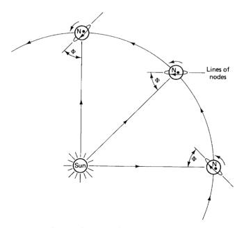
Figure 2.14 Sun-synchronous orbit.
