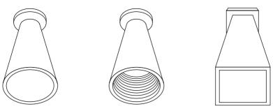
Figure 6.10 Horn antennas: (a) smooth-walled conical, (b) corrugated, and (c) pyramidal.
