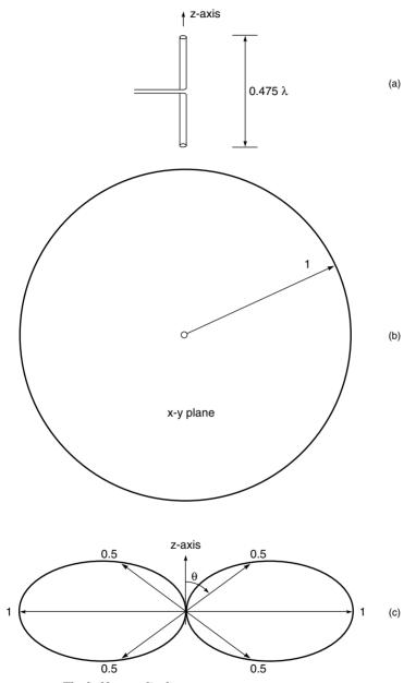
Figure 6.8 The half-wave dipole.
