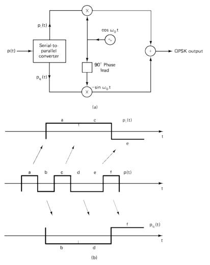
Figure 10.14 (a) QPSK modulator; (b) waveforms for (a).
