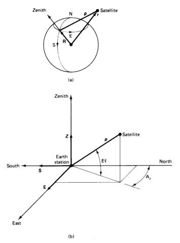
Figure 2.12 Topocentric-horizon coordinate system (SEZ frame): (a) overall view; (b) detailed view.
