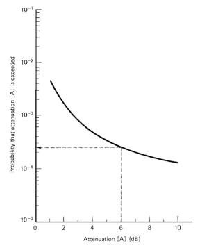
**Figure 12.8** Typical rain attenuation curve used in Ex. (12.17).
