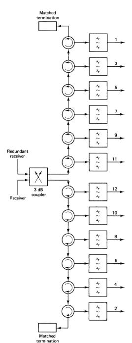
Figure 7.15 Input demultiplexer. (Courtesy of CCIR, CCIR Fixed Satellite Services Handbook, final draft 1984.)
