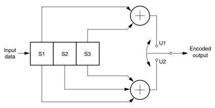
Figure 11.2 A rate 1/2 convolutional encoder.
