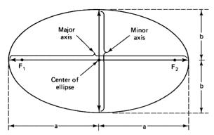
Figure 2.1 The foci  $F_1$  and  $F_2$ , the semimajor axis a, and the semiminor axis b of an ellipse.
