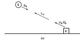
Figure 13.8 (a)Interference modes  $B_1$  and  $B_2$  from network R' into network R. (b) For the  $B_1$  mode the interfering power in dBW/Hz is  $[I_1] = [U_s] + [G'_s] + [G_E] - [L_D]$ . (c) For the  $B_2$  mode the interfering power in dBW/Hz is  $[I_2] = [U_E] + [G'_E] + [G_s] - [L_u]$ .
