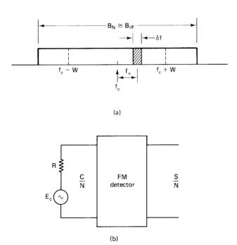
Figure 9.10 (a) The predetector noise bandwidth  $B_{\rm N}$  is approximately equal to the IF bandwidth  $B_{\rm IF}$ . The LF bandwidth W fixes the equivalent postdetector noise bandwidth at 2W.  $\delta f$  is an infinitesimally small noise bandwidth. (b) Receiving system, including antenna represented as a voltage source up to the FM detector.
