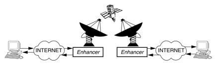
Figure 15.6 Physical architecture incorporating enhancer technology. (From West and McCann, 2000.)
