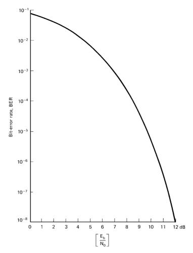
Figure 10.17 BER versus  $(E_{\rm b}/N_{\rm o})$  for baseband signaling using a binary polar NRZ waveform. The curve also applies for BPSK and QPSK modulated waveforms.
