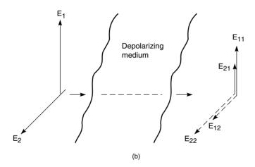
**Figure 5.11** Vectors defining (a) cross-polarization discrimination (XPD) and (b) polarization isolation (I).
