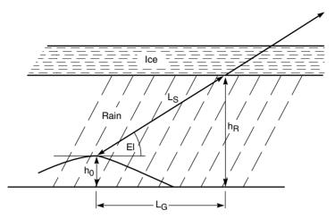
Figure 4.3 Path length through rain.
