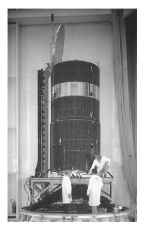
Figure 7.1 The HS 376 satellite. (Courtesy of Hughes Aircraft Company Space and Communications Group.)
