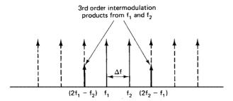
Figure 7.20 Third-order intermodulation products.
