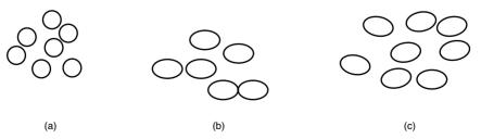
**Figure 5.12** Raindrops: (a) small spherical, (b) flattening resulting from air resistance, and (c) angle of tilt randomized through aerodynamic force.
