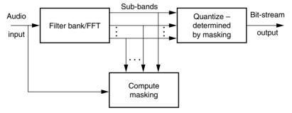
Figure 16.4 MPEG-1 block schematic.
