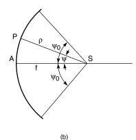
Figure 6.17 (a) The focal length f = SA and a ray path SPQ. (b) The focal distance  $\rho$ .
