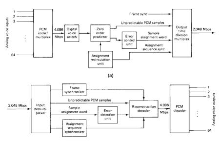
Figure 14.23 (a) SPEC transmitter, (b) SPEC receiver. (From Sciulli and Campanella, 1973. © 1973—IEEE.)
