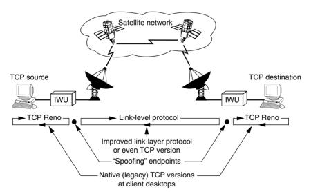
Figure 15.5 TCP/IP satellite link spoofing configuration. (From Ghani and Dixit, 1999. © 1999 IEEE.)
