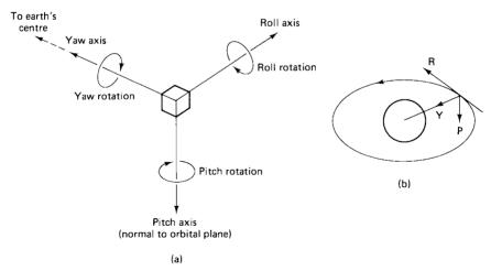
**Figure 7.4** (a) Roll, pitch, and yaw axes. The yaw axis is directed toward the earth's center, the pitch axis is normal to the orbital plane, and the roll axis is perpendicular to the other two. (b) RPY axes for the geostationary orbit. Here, the roll axis is tangential to the orbit and lies along the satellite velocity vector.
