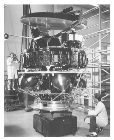
Figure 7.7 Technicians check the alignment of the Telestar 3 communications satellite, shown without its cylindrical panels. The satellite, built for the American Telephone and Telegraph Co., carries both traveling-wave tube and solid-state power amplifiers, as shown on the communications shelf surrounding the center of the spacecraft. The traveling-wave tubes are the cylindrical instruments. (Courtesy of Hughes Aircraft Company Space and Communications Group.)
