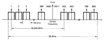
Figure 14.5 Channeling arrangement for Intelsat SCPC system.
