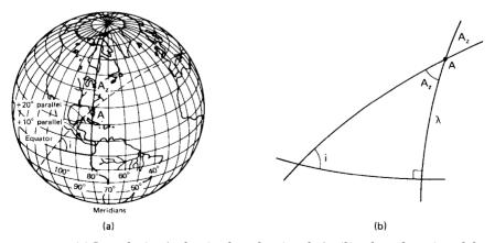
Figure 3.13 (a) Launch site A, showing launch azimuth  $A_z$ ; (b) enlarged version of the spherical triangle shown in (a).  $\lambda$  is the latitude of the launch site.
