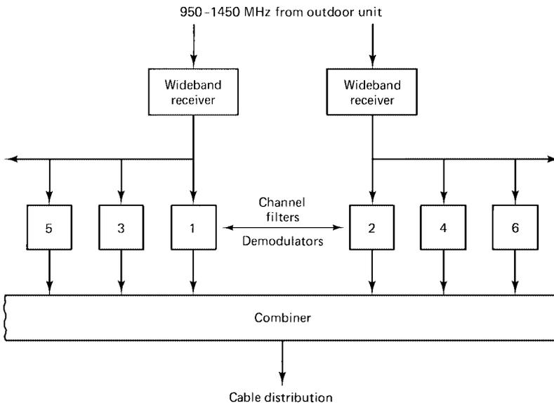
**Figure 8.3** One possible arrangement for the indoor unit of a community antenna TV (CATV) system.
