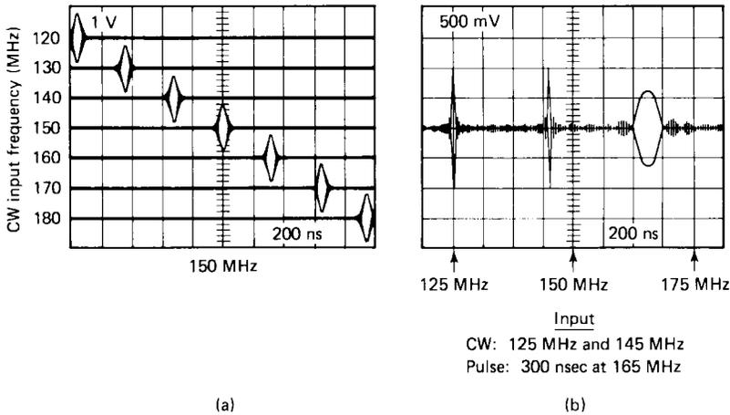
**Figure 14.26** Prototype chirp transform of (a) seven successive CW input signals and (b) three simultaneous input signals, including CW and pulsed RF. 200 ns/div; 31.5 MHz/ $\mu$ s chirp rate. (From Hays and Hartmann, 1976. © 1976—IEEE.)
