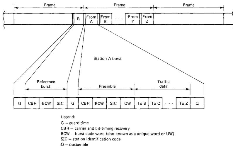
Figure 14.13 Frame and burst formats for a TDMA system.
