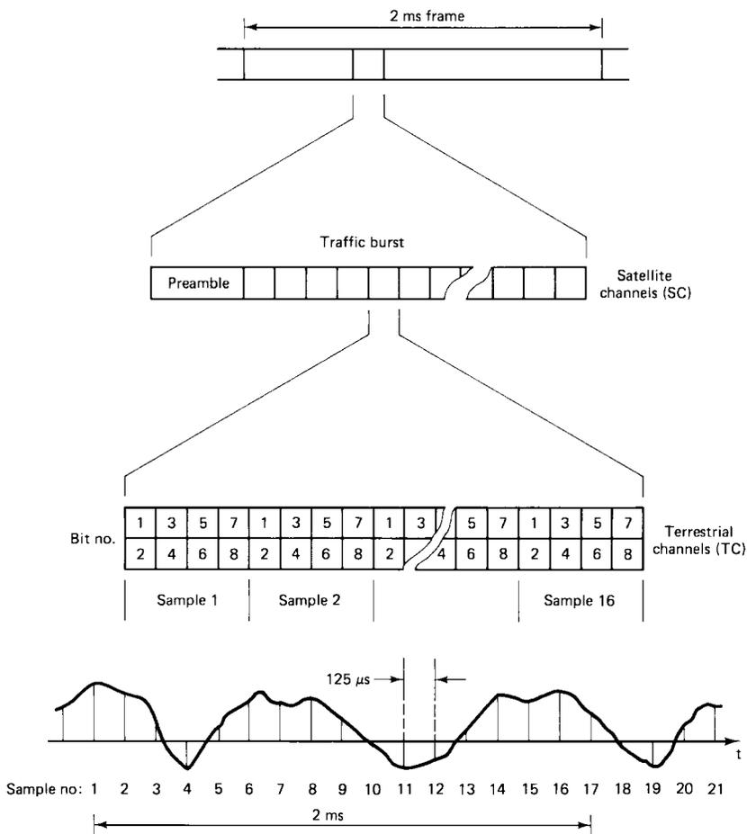
Figure 14.20 Preassigned TDMA frame in the Intelsat system.
