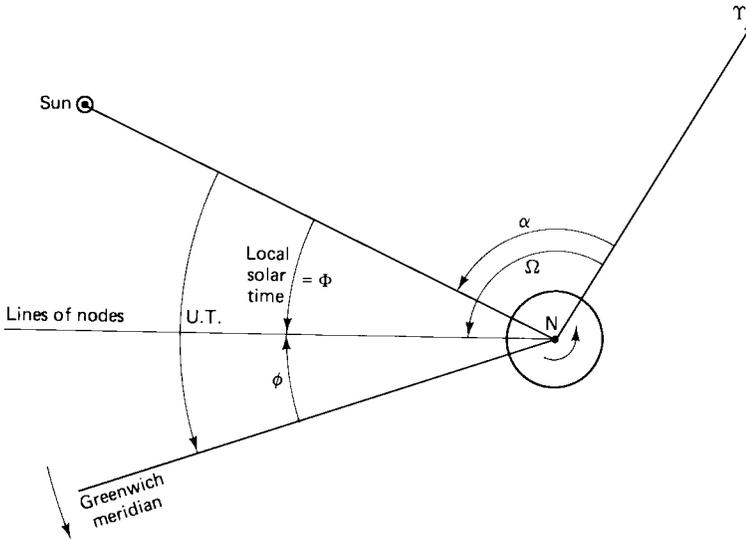
**Figure 2.15** The condition for sun synchronicity is that the local solar time should be constant. Local solar time =  $\Omega - \alpha$ , which is also equal to the angle  $\Phi$  shown in Fig. 2.14. This is the local solar time at the ascending node, but a similar situation applies at other latitude crossings.
