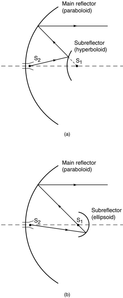
**Figure 6.23** Ray paths for (a) Cassegrain and (b) Gregorian antennas.
