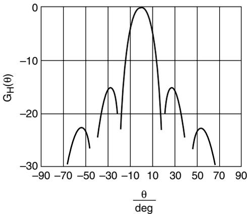
The results of Example 6.1 show the main lobe and the sidelobes. These are a general feature of aperture antennas, and as mentioned above, the pattern is the result of interference phenomena. Mathematically, the lobes result from the  $(\sin X)/X$  and  $(\sin Y)/Y$  terms. One of the main concerns in satellite communications is the reduction of interference caused by sidelobes.
