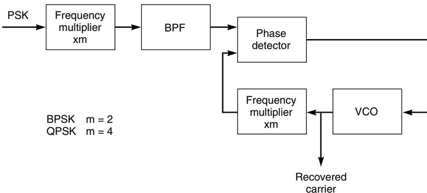
Figure 10.20 Functional block diagram for carrier recovery.
