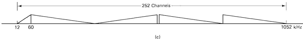
**Figure 9.4** Examples of baseband signals for FDM telephony: (a) 24 channels; (b) 60 channels; (c) 252 channels.
