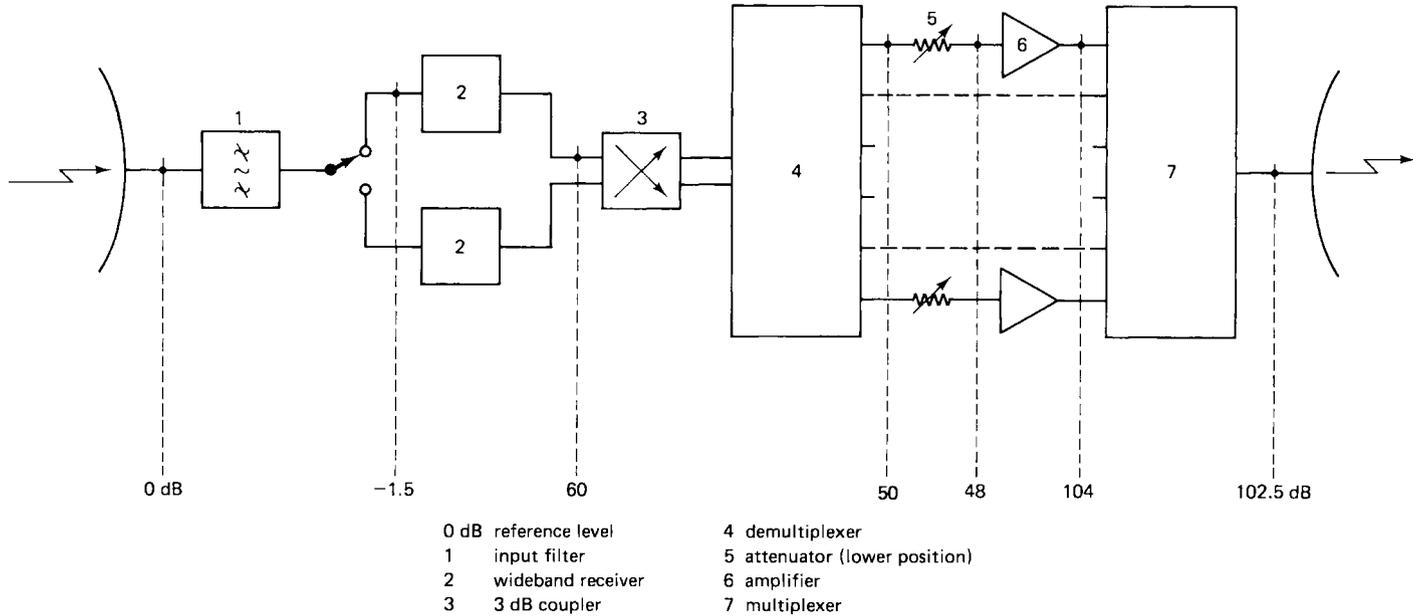
**Figure 7.16** Typical diagram of the relative levels in a transponder. (Courtesy of CCIR, *CCIR Fixed Satellite Services Handbook, final draft 1984.*)
