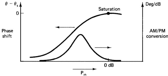
**Figure 7.19** Phase characteristics for a TWT.  $\theta$  is the input-to-output phase shift, and  $\theta_s$  is the value at saturation. The AM/PM curve is derived from the slope of the phase shift curve.
