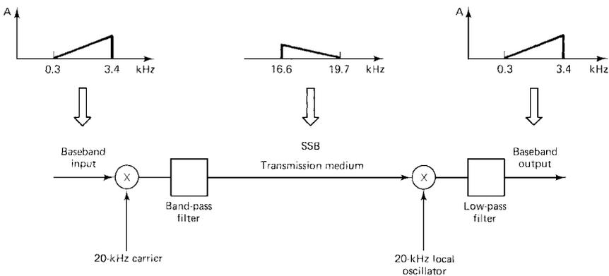
**Figure 9.2** A basic SSB transmission scheme.
