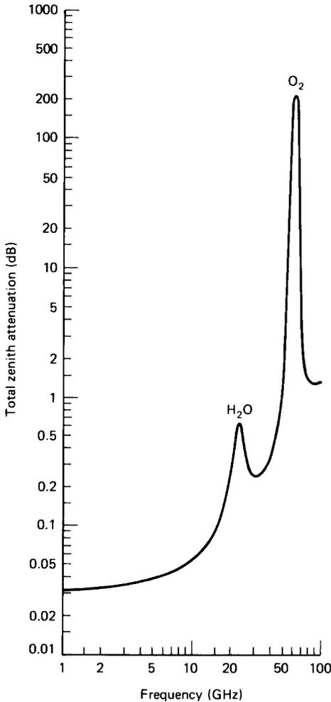
**Figure 4.2** Total zenith attenuation at ground level: pressure = 1 atm, temperature = 20°C, and water vapor = 7.5 g/m<sup>3</sup>. (Adapted from CCIR Report 719-2, with permission from International Telecommunication Union.)
