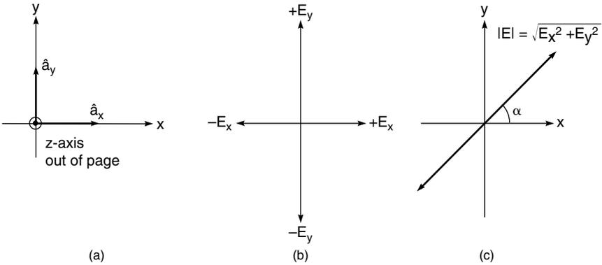
**Figure 5.2** Horizontal and vertical components of linear polarization.
