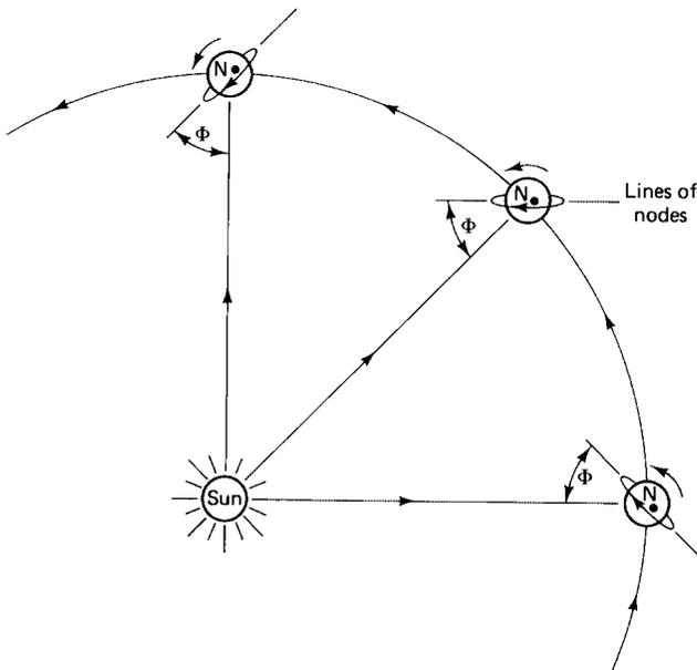
Figure 2.14 Sun-synchronous orbit.
