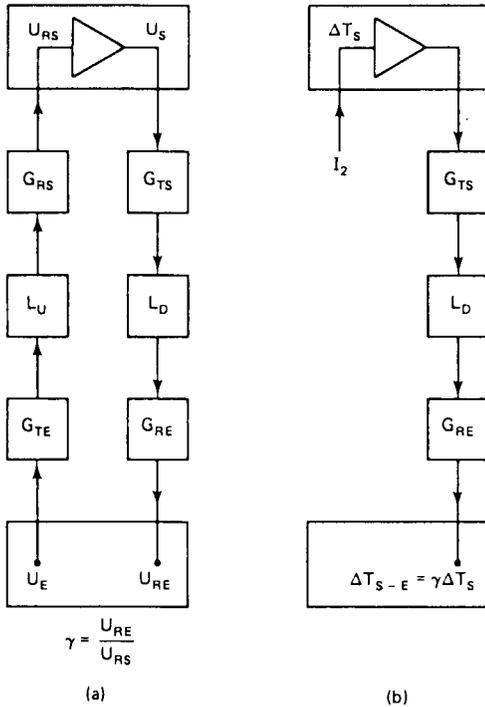
**Figure 13.9** (a) Defining the transmission gain  $\gamma$  in Sec. 13.4.2. (b) Use of transmission gain to refer satellite noise temperature to an earth-station.
