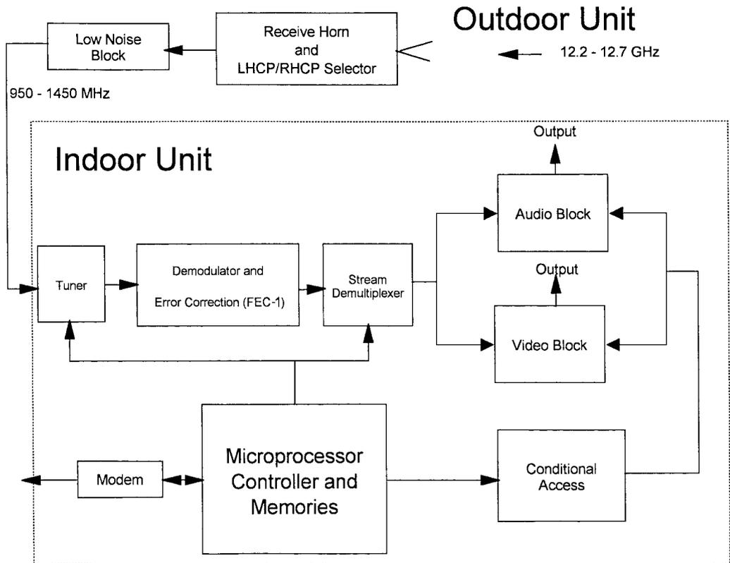
Figure 16.7 Block schematic for the indoor unit (IDU).
