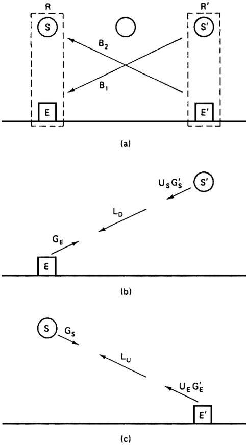
**Figure 13.8** (a) Interference modes  $B_1$  and  $B_2$  from network  $R'$  into network  $R$ . (b) For the  $B_1$  mode the interfering power in dBW/Hz is  $[I_1] = [U_s] + [G'_s] + [G_E] - [L_D]$ . (c) For the  $B_2$  mode the interfering power in dBW/Hz is  $[I_2] = [U_E] + [G'_E] + [G_s] - [L_u]$ .
