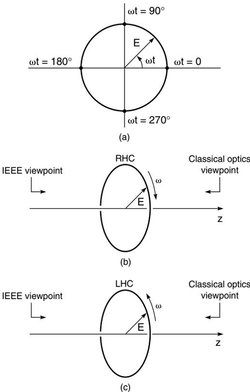
Figure 5.3 Circular polarization.
