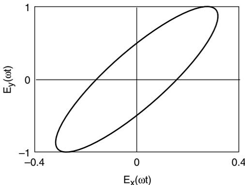
**Figure 5.4** Elliptical polarization.
