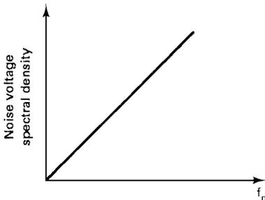
Figure 9.11 Noise voltage spectral density for FM.
