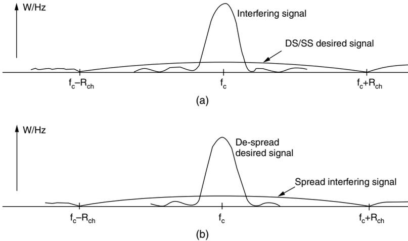
**Figure 14.39** (a) Spectrum of an interfering, nonspread signal along with the spread desired signal; (b) the effect of the de-spreading operation on the desired signal resulting in spread of the interferer.
