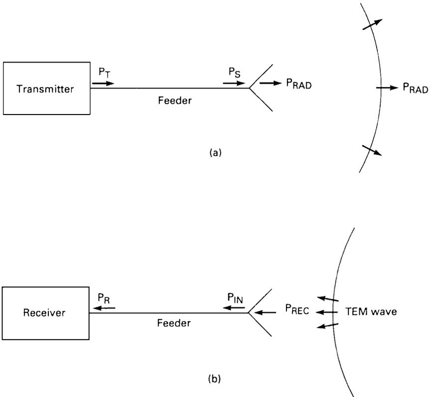
Figure 6.1 (a) Transmitting antenna. (b) Receiving antenna.
