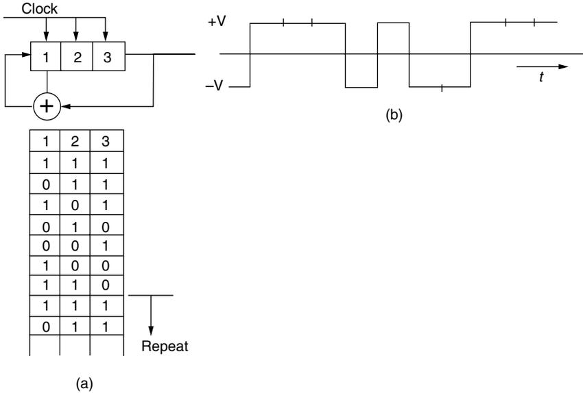
**Figure 14.34** Generation of a 7-chip maximal sequence code.
