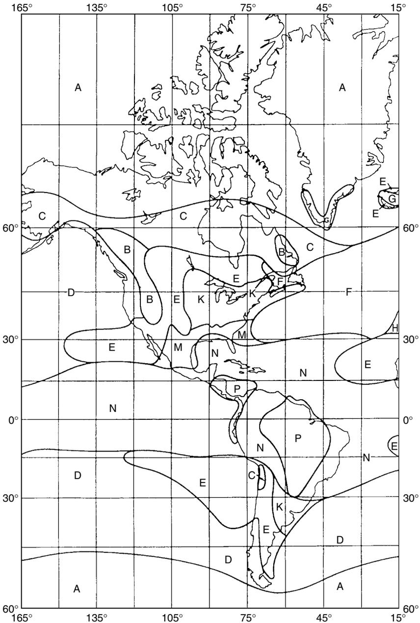
**Figure 16.8** Rain climatic zones. Refer to Table 16.2. (From Rec. ITU-R PN.837-1, with permission from the copyright holder ITU. Sole responsibility for the reproduction rests with the author. The complete volume of the ITU material from which the material is extracted can be obtained from the International Telecommunication Union, Sales and Marketing Service, Place des Nations-CH-1211, Geneva 20, Switzerland.)
