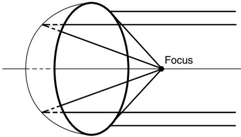
**Figure 6.16** The focusing property of a paraboloidal reflector.
