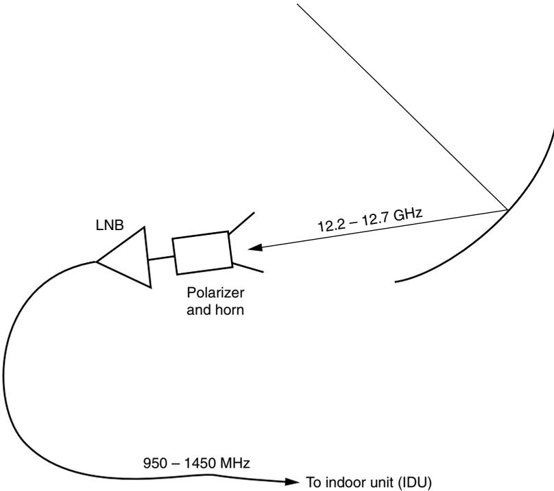
Figure 16.5 Block schematic for the outdoor unit (ODU).
