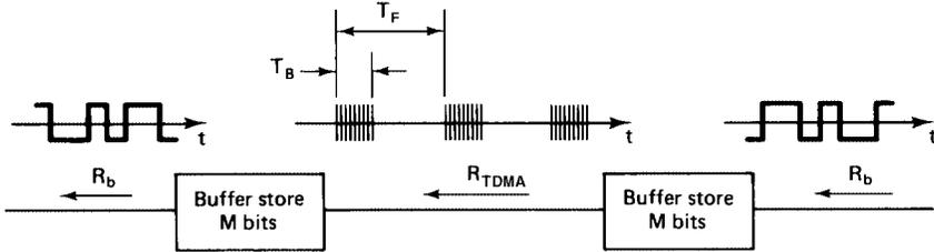
Figure 14.11 Burst-mode transmission linking two continuous-mode streams.
