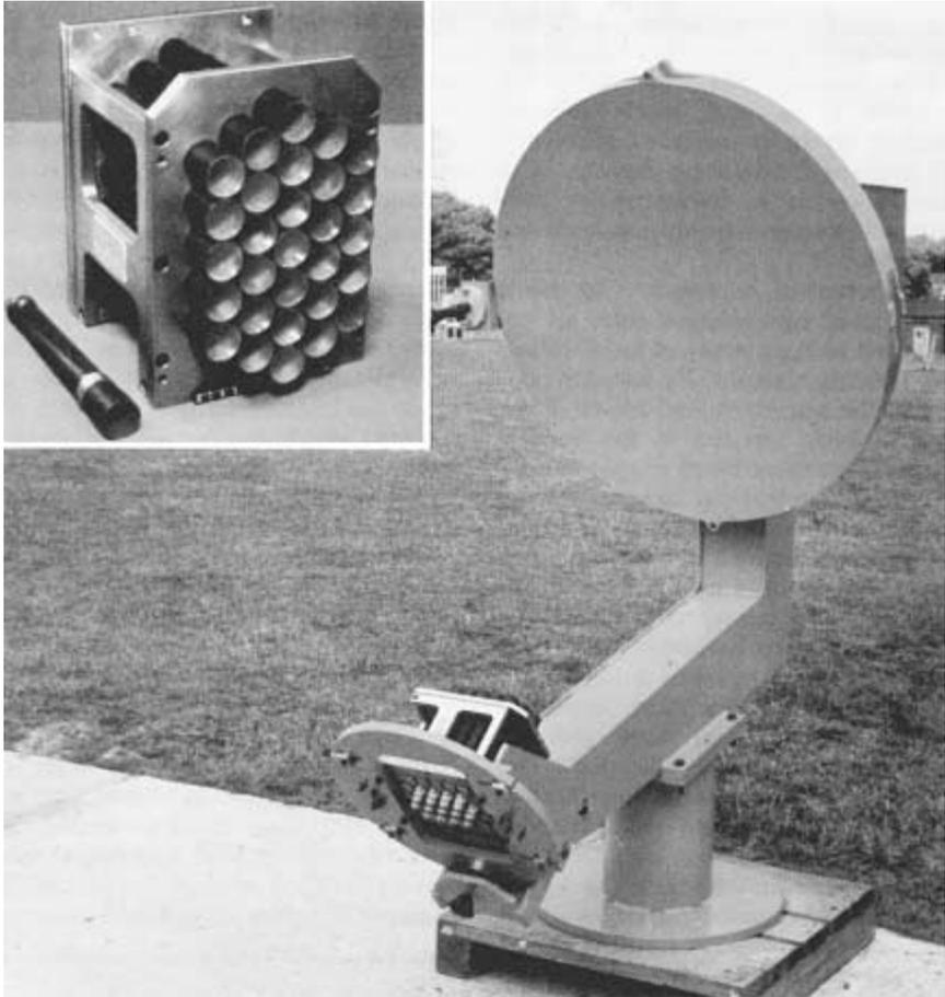
**Figure 6.28** A multifeed contained-beam reflector antenna. (From Brain and Rudge, 1984, with permission.)
