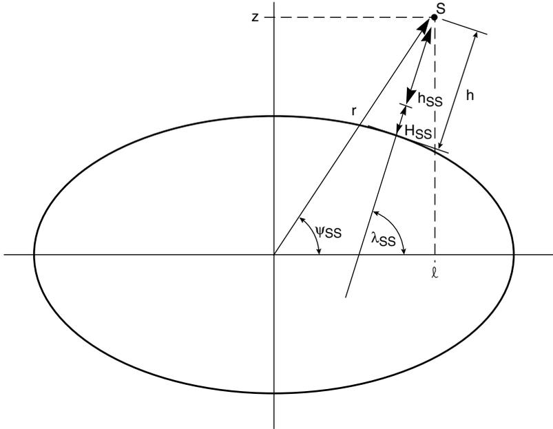
**Figure 2.13** Geometry for determining the subsatellite point.
