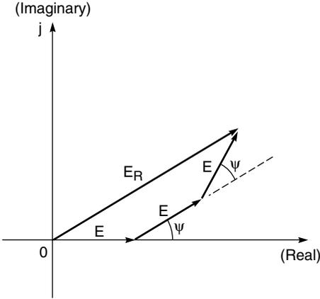
Figure 6.27 Phasor diagram for the in-line array of dipoles.
