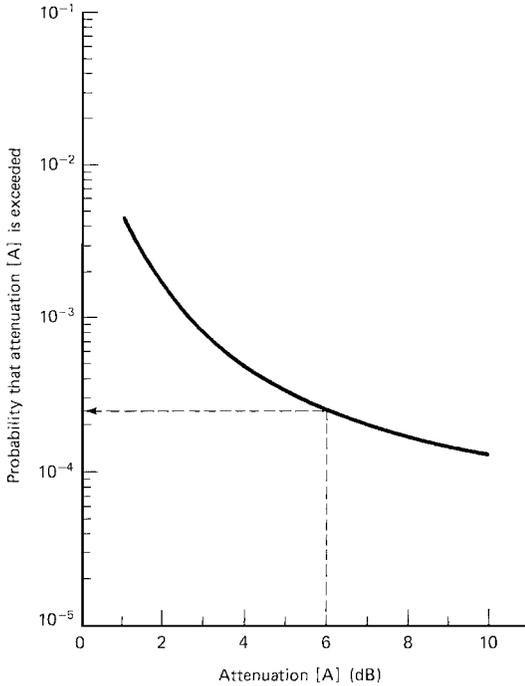
**Figure 12.8** Typical rain attenuation curve used in Ex. (12.17).
