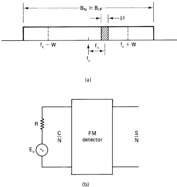
**Figure 9.10** (a) The predetector noise bandwidth  $B_N$  is approximately equal to the IF bandwidth  $B_{IF}$ . The LF bandwidth  $W$  fixes the equivalent postdetector noise bandwidth at  $2W$ .  $\delta f$  is an infinitesimally small noise bandwidth. (b) Receiving system, including antenna represented as a voltage source up to the FM detector.
