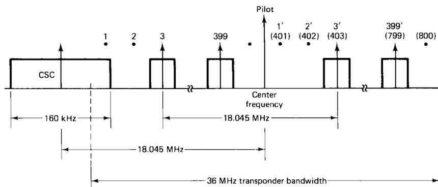
Figure 14.8 Channeling scheme for the Spade system.
