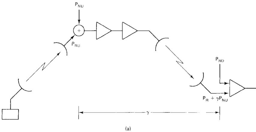
Figure 12.9 (a) Combined uplink and downlink; (b) power flow diagram for (a).
