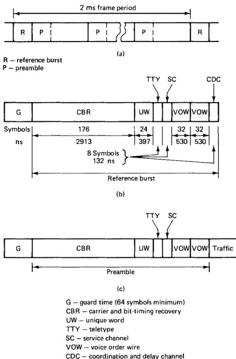
Figure 14.14 (a) IntelSat 2-ms frame; (b) composition of the reference burst *R*; (c) composition of the preamble *P*. (QPSK modulation is used, giving 2 bits per symbol. Approximate time intervals are shown.)
