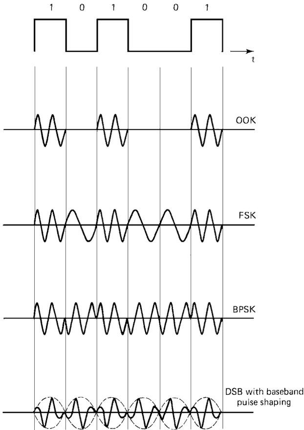
Figure 10.11 Some binary digital modulation formats.
