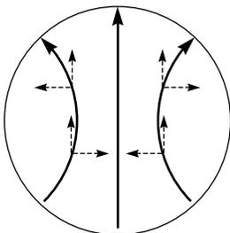
**Figure 6.11** Aperture field in a smooth-walled conical horn.
