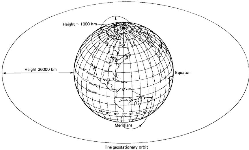
**Figure 1.6** Geostationary orbit and one possible polar orbit.
