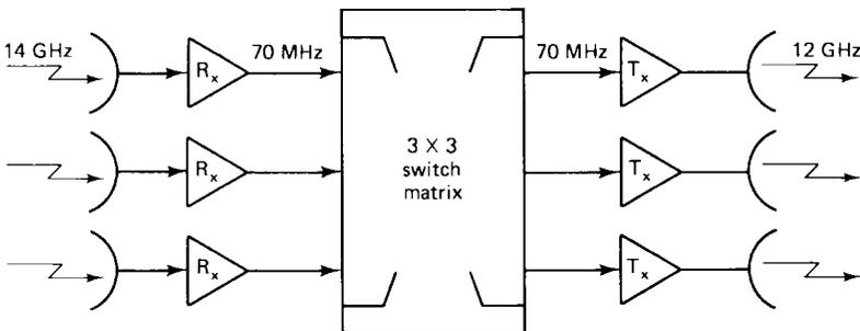
Figure 14.28 Switch matrix in the R.F. link.
