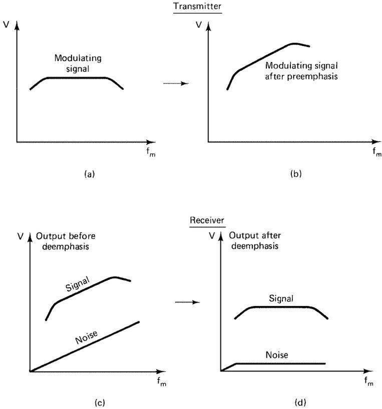
**Figure 9.13** (a) and (b) Effect of preemphasis on the modulating signal frequency response at the transmitter. (c) and (d) Effect of deemphasis on the modulating signal and noise at the receiver output. The deemphasis cancels out the preemphasis for the signal while attenuating the noise at the receiver.
