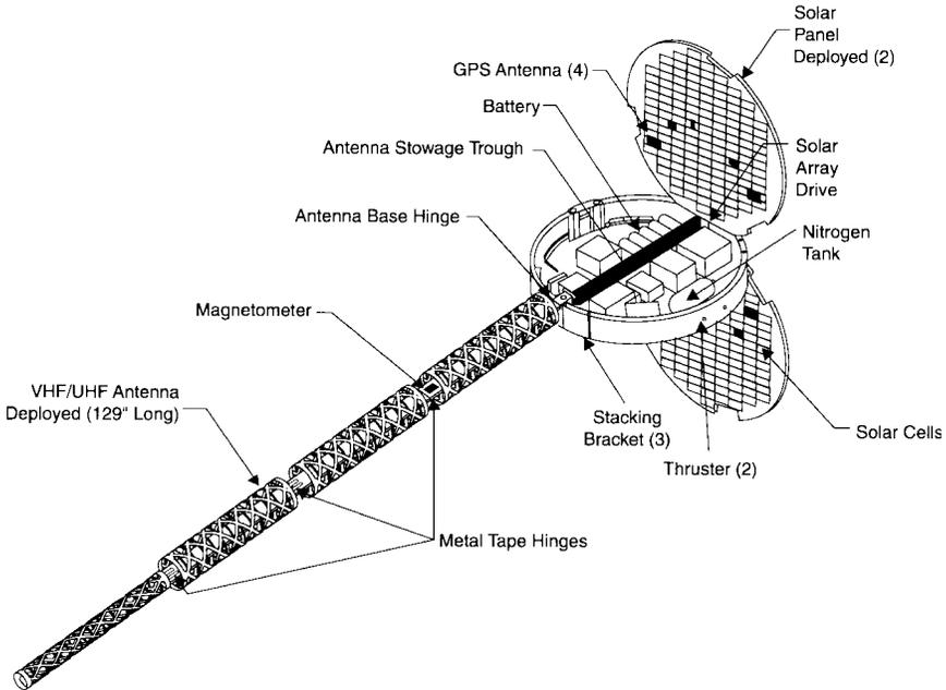
**Figure 17.5** Orbcomm/Microstar satellite. (Courtesy Orbital Communications Corporation.)
