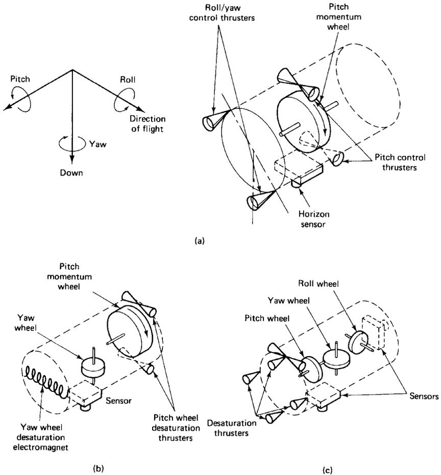
**Figure 7.8** Alternative momentum wheel stabilization systems: (a) one-wheel; (b) two-wheel; (c) three-wheel. (Reprinted with permission from *Spacecraft Attitude Determination and Control*, edited by James R. Wertz. Copyright © 1984 by D. Reidel Publishing Company, Dordrecht, Holland.)
