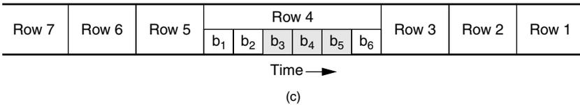
Figure 11.5 Illustrating interleaving (see Sec. 11.5).
