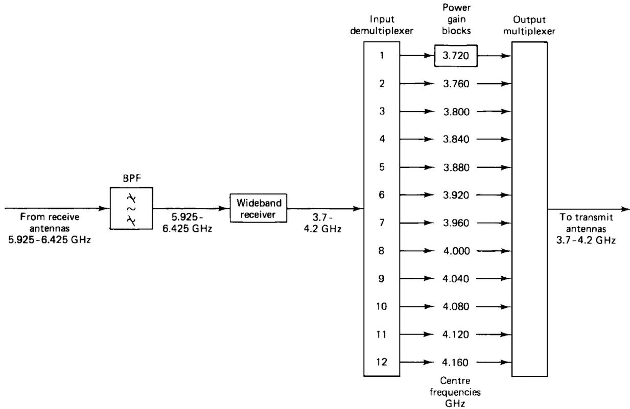
**Figure 7.13** Satellite transponder channels. (Courtesy of CCIR, *CCIR Fixed Satellite Services Handbook, final draft 1984.*)
