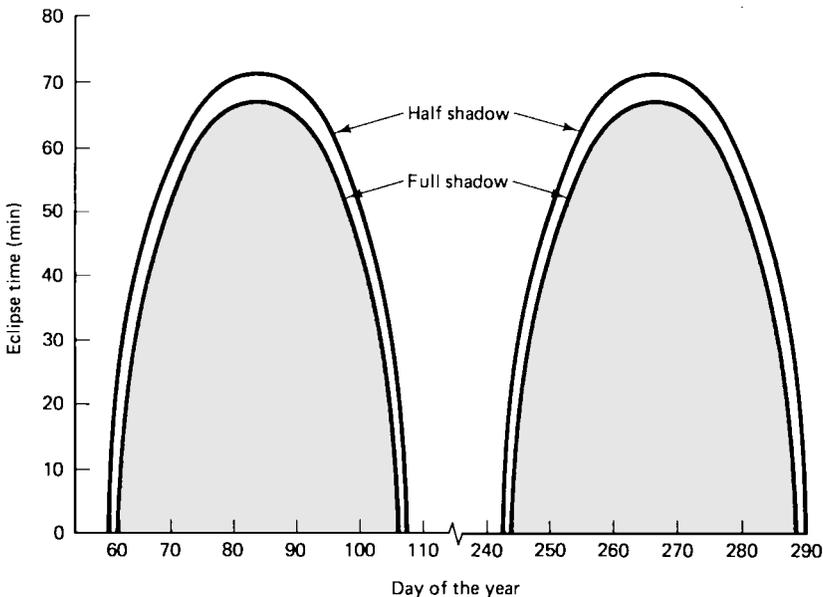
**Figure 7.3** Satellite eclipse time as a function of the current day of the year. (From Spilker, 1977. Reprinted by permission of Prentice-Hall, Englewood Cliffs, NJ.)
