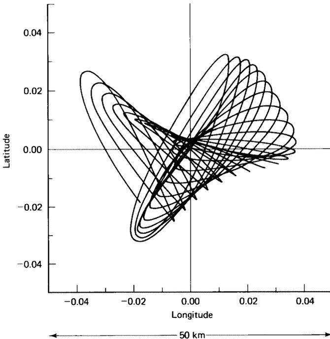
**Figure 7.9** Typical satellite motion. (From *Telesat, Canada, 1983*; courtesy of Telesat Canada.)
