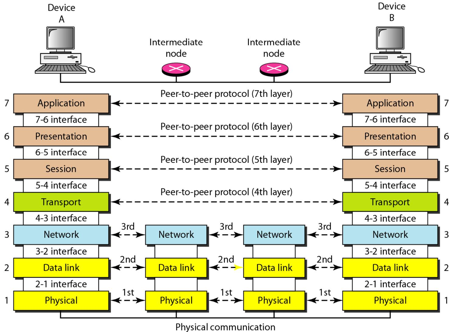
**Figure 2.4** *An exchange using the OSI model*
