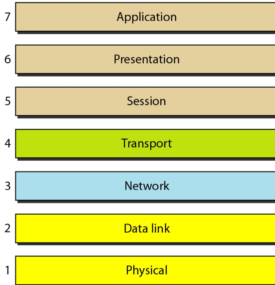
**Figure 2.3** *The interaction between layers in the OSI model*
