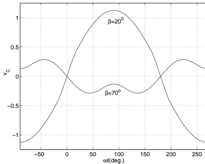
Figure 4.9: Capacitor voltage waveforms for  $\beta = 20^\circ$   $\beta = 70^\circ$
