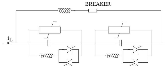
Figure 4.3: Single Line Diagram of a TCSC
