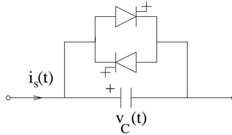
Figure 4.15: GTO Controlled Series Capacitor (GCSC)
