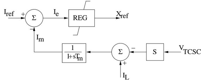
Figure 4.12: Block diagram of CC or CA controller
