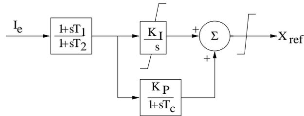
Figure 4.13: Block diagram of the Regulator
