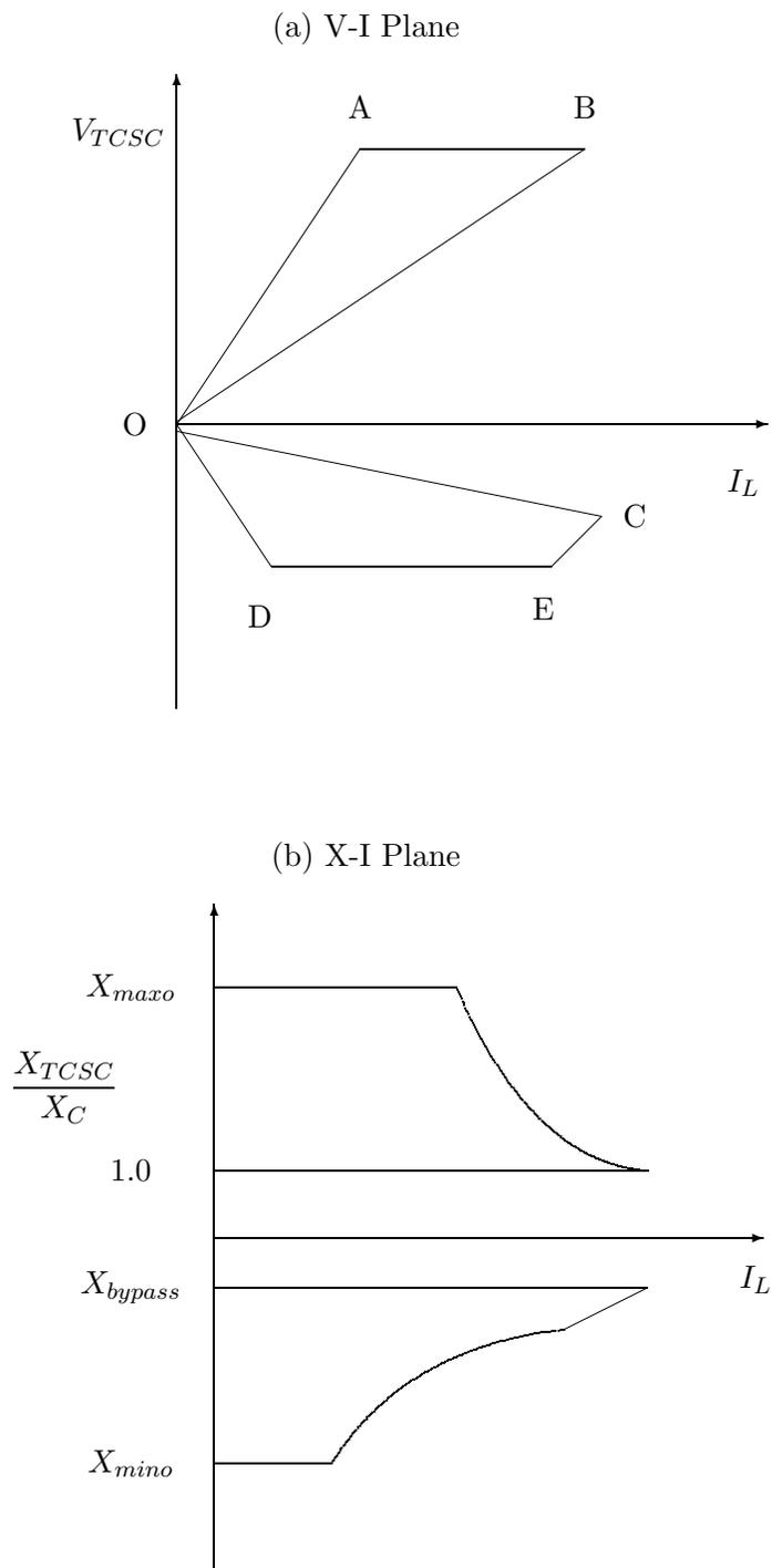
Figure 4.14: TCSC capability curves for a module
