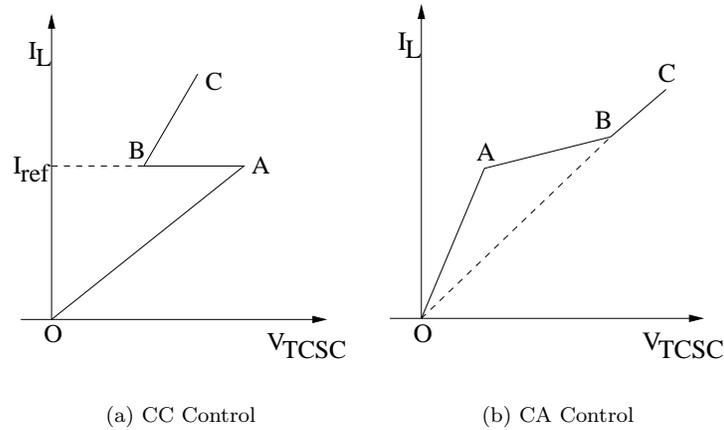
Figure 4.10: Control Characteristics
