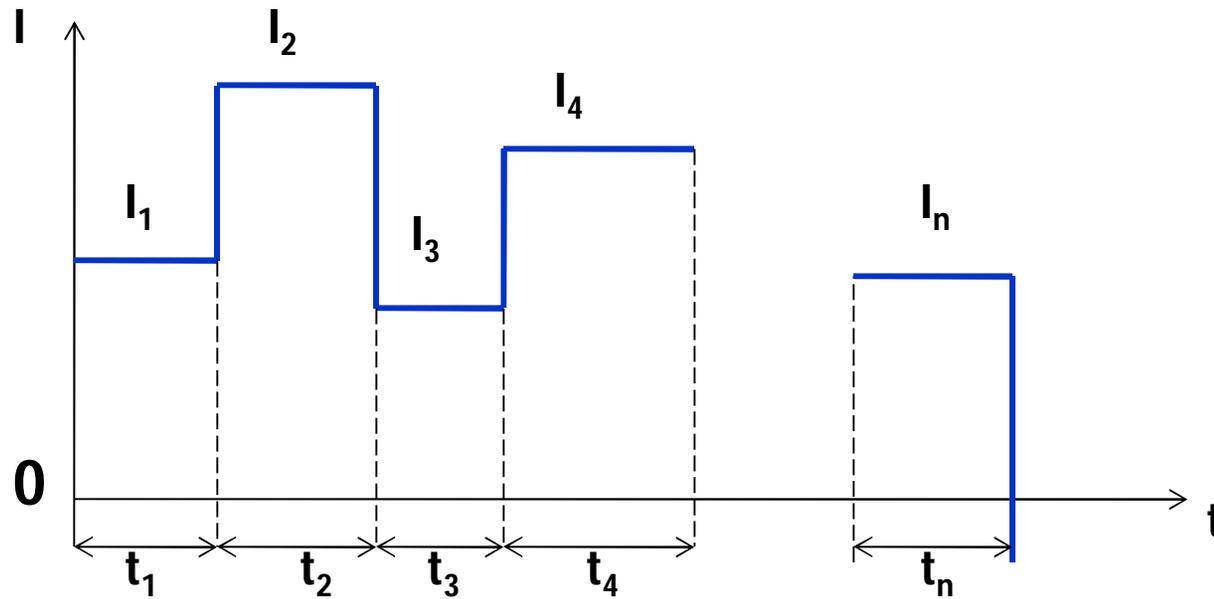
**Fig. 5.5. (a) Load diagram of Fluctuating load**
