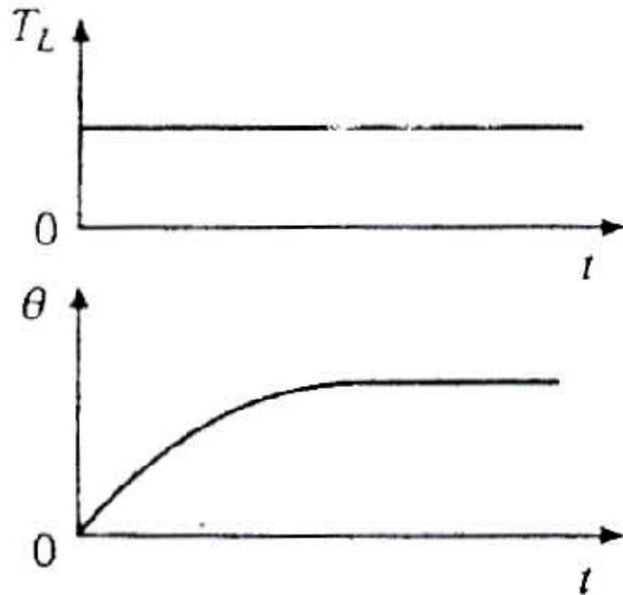
It denotes the motor operation at a constant load torque for a duration long enough for the motor temperature to reach steady state value. This duty is characterized by a constant motor loss.
