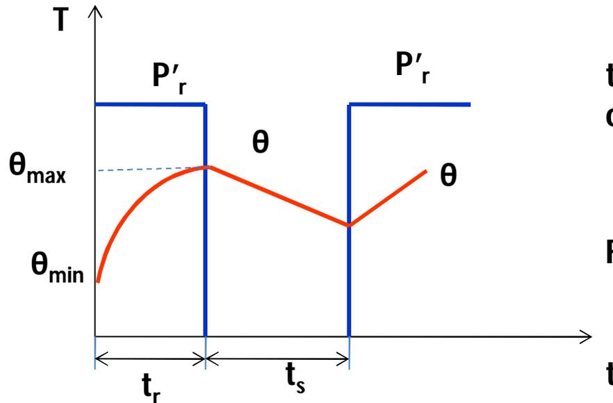
$t_r$  and  $t_s$  are thermal time constants of motor for working and standstill
