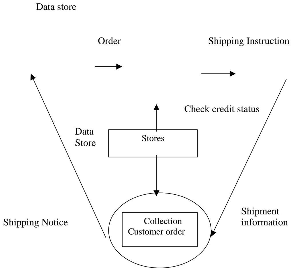
Fig. 7.16 Data flow diagram for order processing and shipping for a publishing company.
