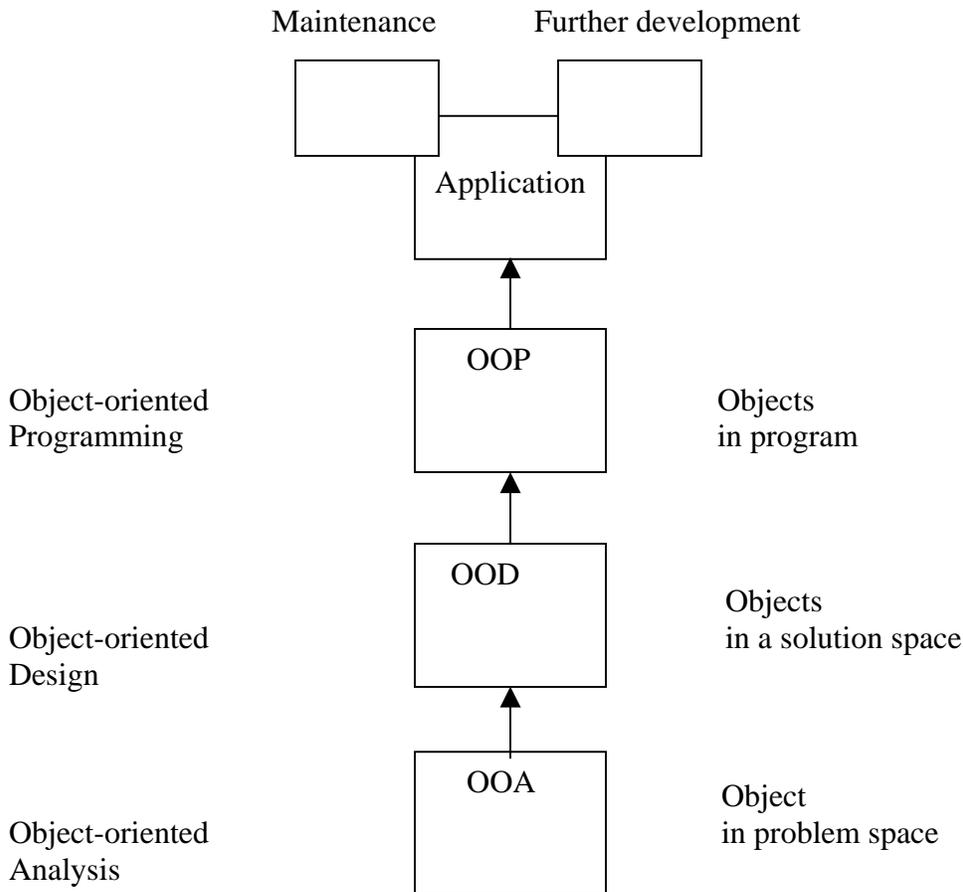
Fig. 7.4 Fountain model of object-oriented software development
