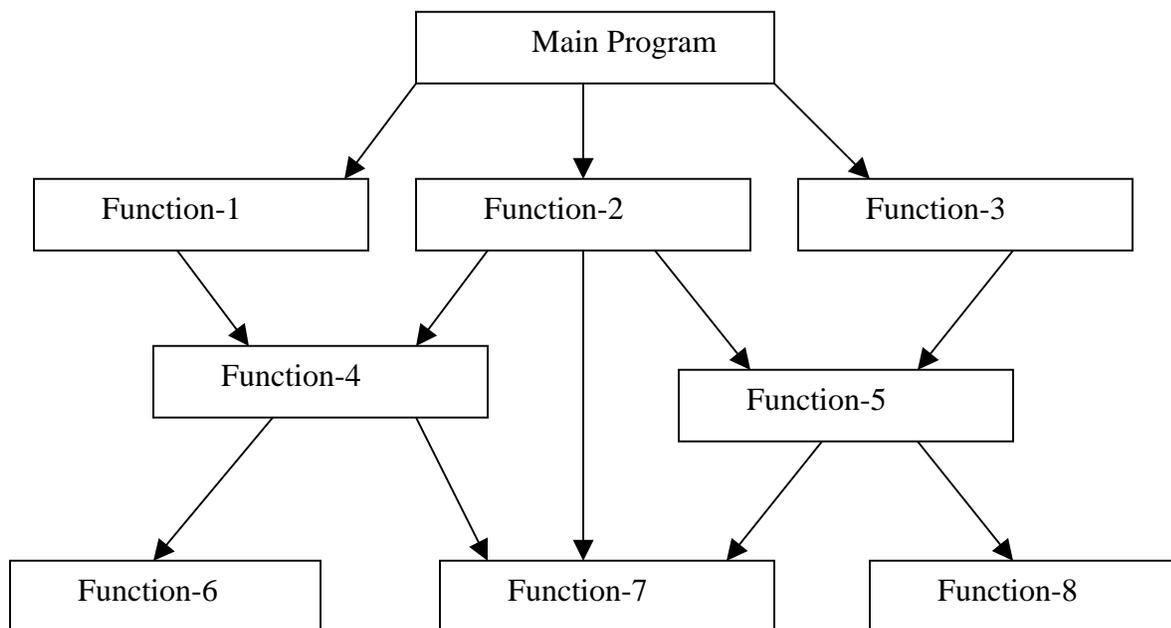
Fig. 1.2 Typical structure of procedural oriented programs
