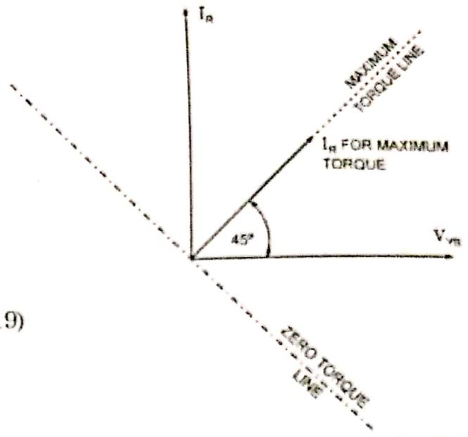
Phasor Diagram For  $90^\circ$  Directional Relay With  $45^\circ$  Maximum Torque Angle
