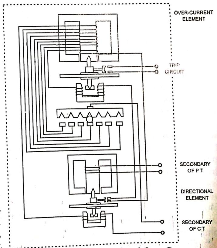
*Induction Type Directional Over-Current and Earth-Fault Relay*
