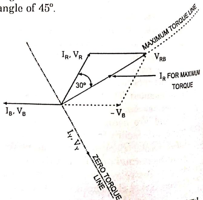
Phasor Diagram For  $0^\circ$  Directional Relay With Zero Maximum Torque Angle
