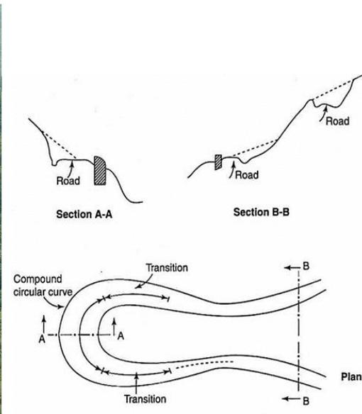
Schematic dig. of hair pin bend curve
