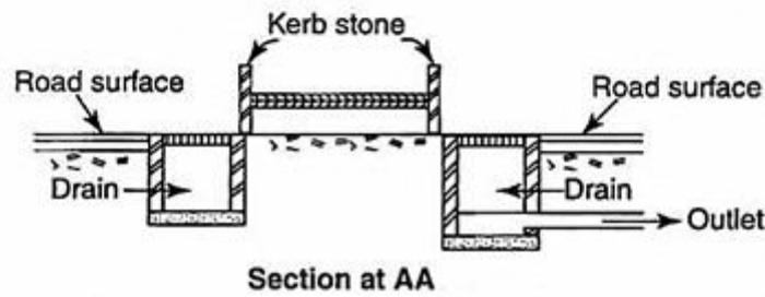
Fig. Typical drainage arrangement at a Rotary
