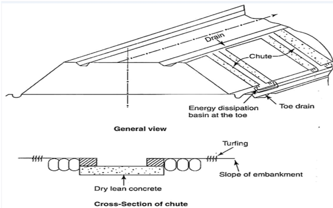
Fig. Drainage system for high Embankment
