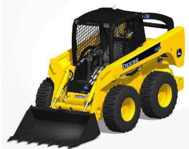
Fig. Skid steer loader
