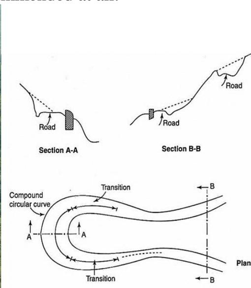
Schematic dig. of hair pin bend curve
