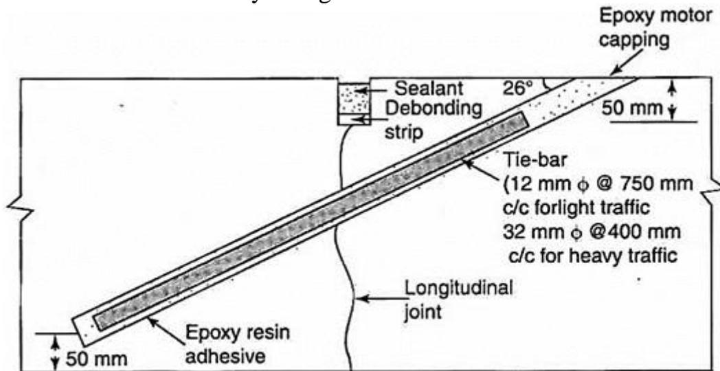
**FIG. 10.9** Crack repair by cross-stitching
