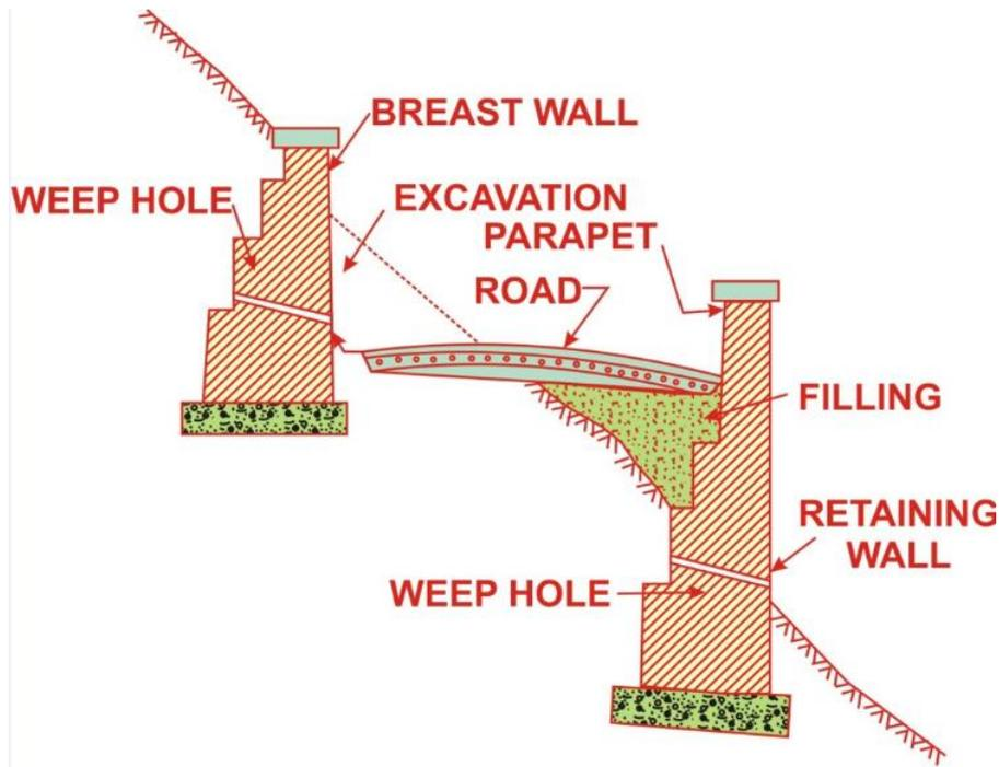
Fig. Retaining wall and breast wall
