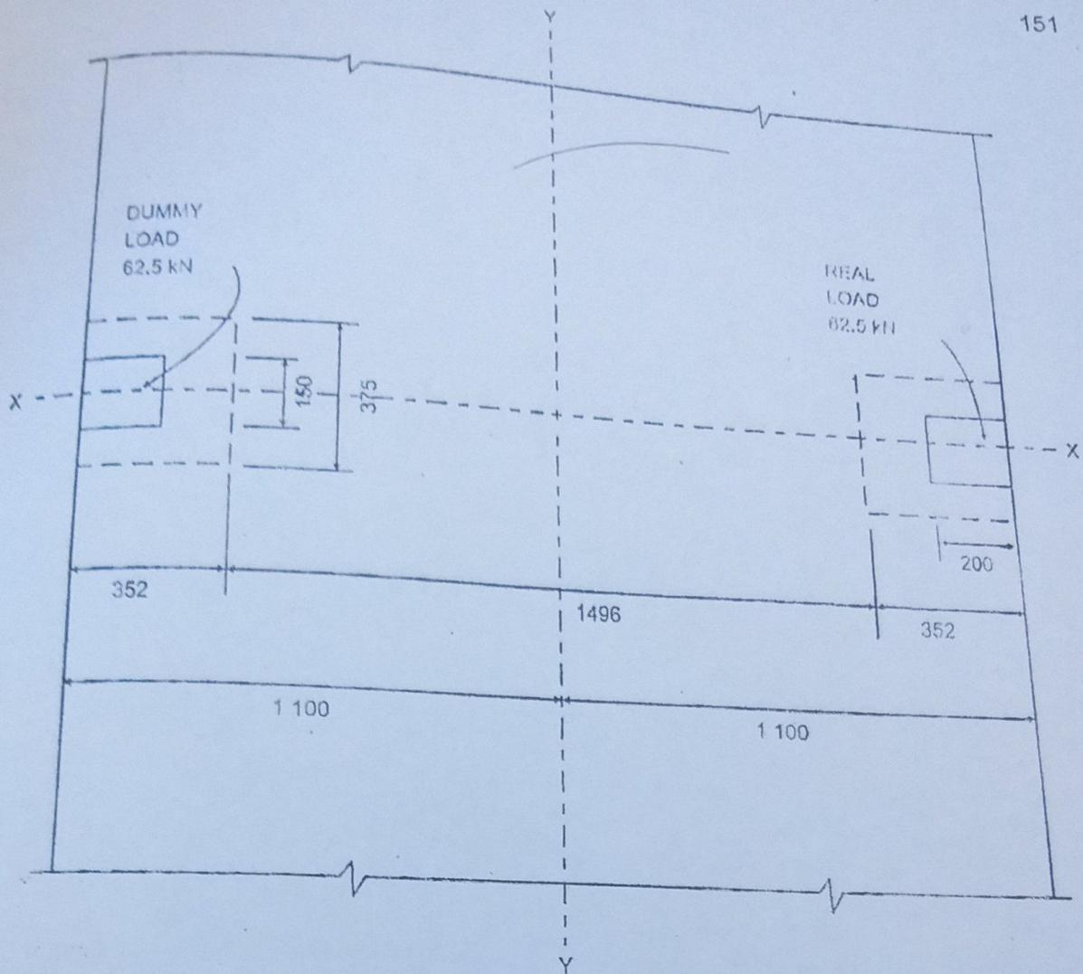
Figure 7.6 Details of Disposition of Wheel 2.
