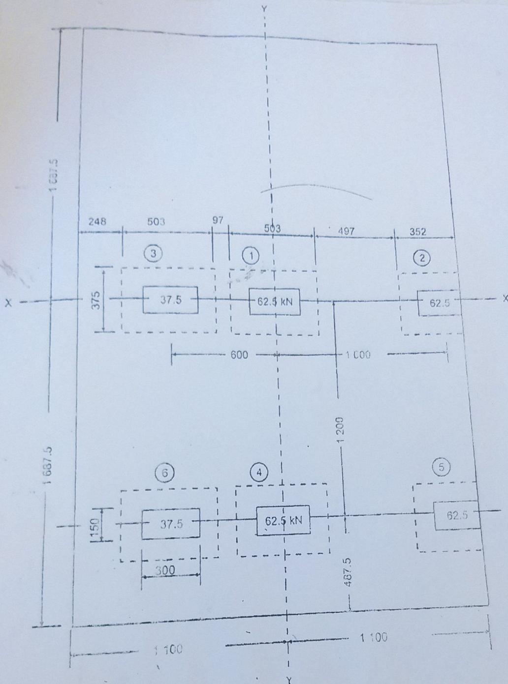
Figure 7.5 Disposition of Class AA Wheeled Vehicle for Maximum Moment.
