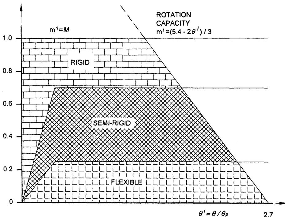
**FIG. 33 CLASSIFICATION OF CONNECTIONS ACCORDING TO BJORHOVDE**
