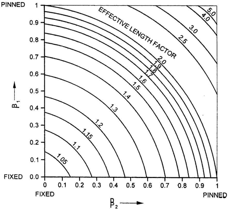
FIG. 28 COLUMN EFFECTIVE LENGTH FACTOR — SWAY FRAME
