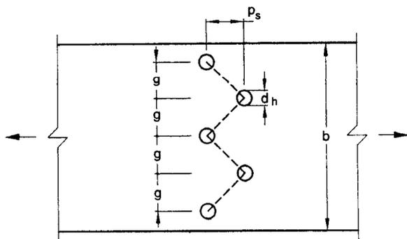
FIG. 5 PLATES WITH BOLTS HOLES IN TENSION
