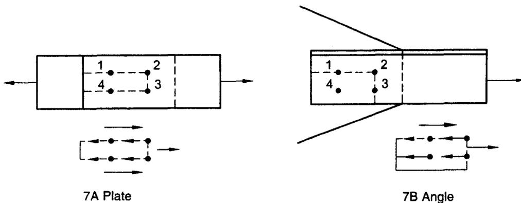
FIG. 7 BLOCK SHEAR FAILURE
