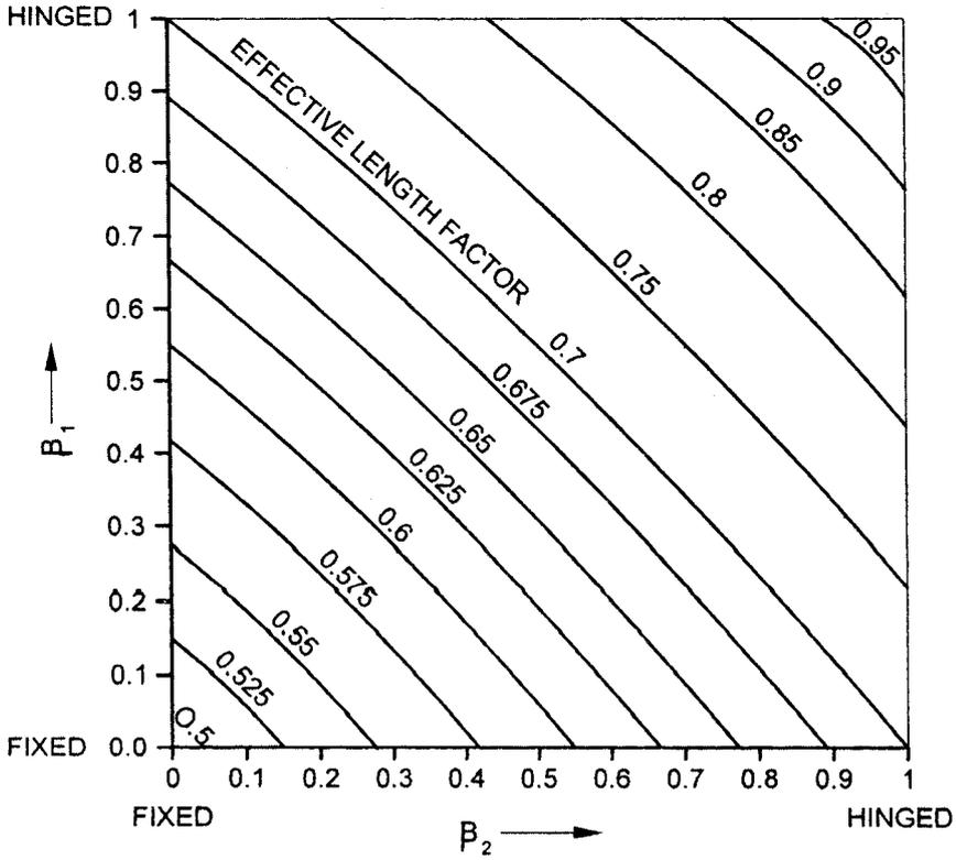
FIG. 27 COLUMN EFFECTIVE LENGTH FACTOR — NON-SWAY FRAME
