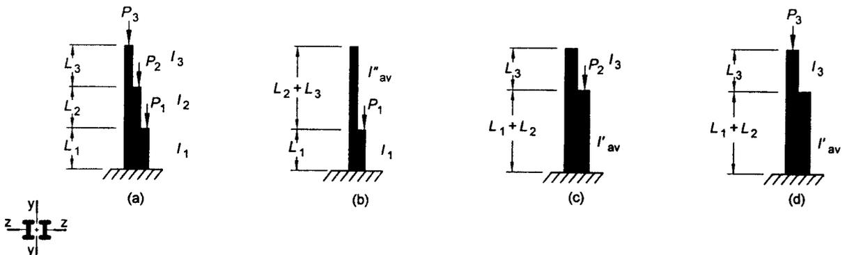
FIG. 29 EFFECTIVE LENGTH OF DOUBLE STEPPED COLUMNS
