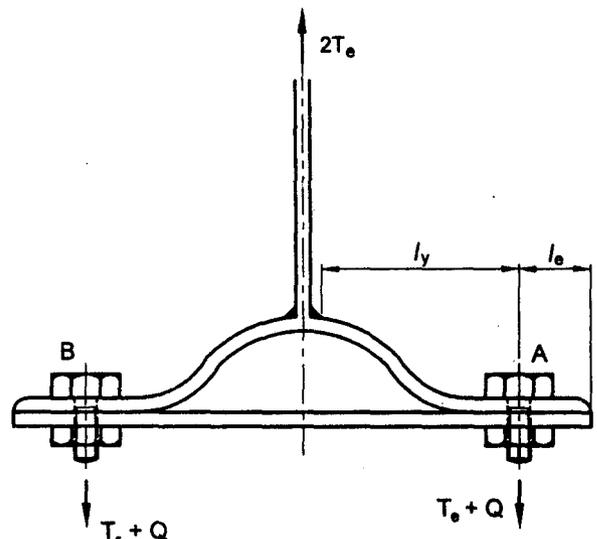
FIG. 16 COMBINED PRYING FORCE AND TENSION
