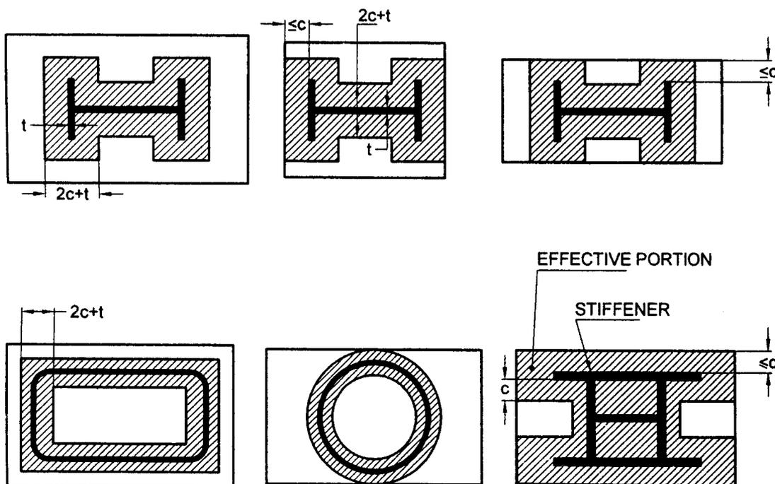
FIG. 9 EFFECTIVE AREA OF A BASE PLATE
