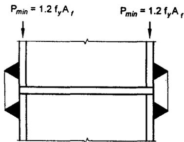
FIG. 20 PARTIAL PENETRATION GROOVE WELD IN COLUMN SPLICE
