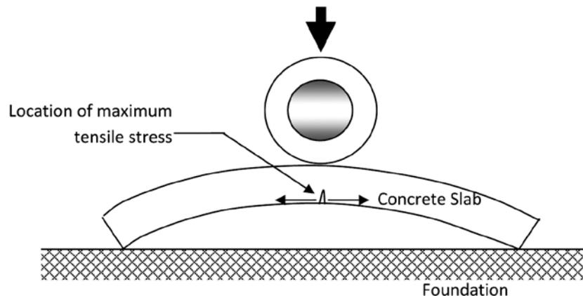
Fig. 3 Axle Load Placed in the Middle of the Slab during Mid-Day
