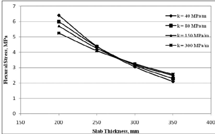
Fig. IV.25 Stress due to Single Axle Load of 200 kN, ΔT = 21°C, Without Concrete Shoulder
