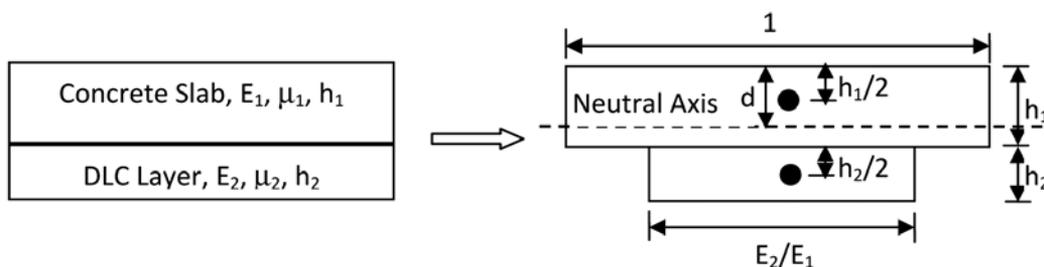
Fig. 7 Concept used for Obtaining Combined Flexural Stiffness
