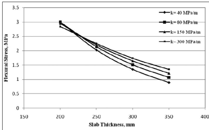
Fig. IV.17 Stress due to Single Axle Load of 80 kN,  $\Delta T = 17^\circ\text{C}$ , Without Concrete Shoulder
