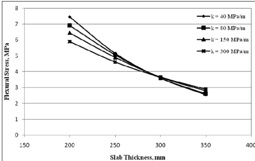
Fig. IV.26 Stress due to Single Axle Load of 240 kN, ΔT = 21°C, Without Concrete Shoulder
