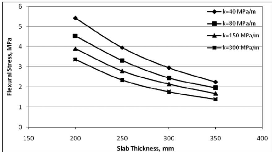
Fig. IV.57 Stress due to Tandem Axle Load of 480 kN,  $\Delta T = 0^\circ\text{C}$ , Without Concrete Shoulder
