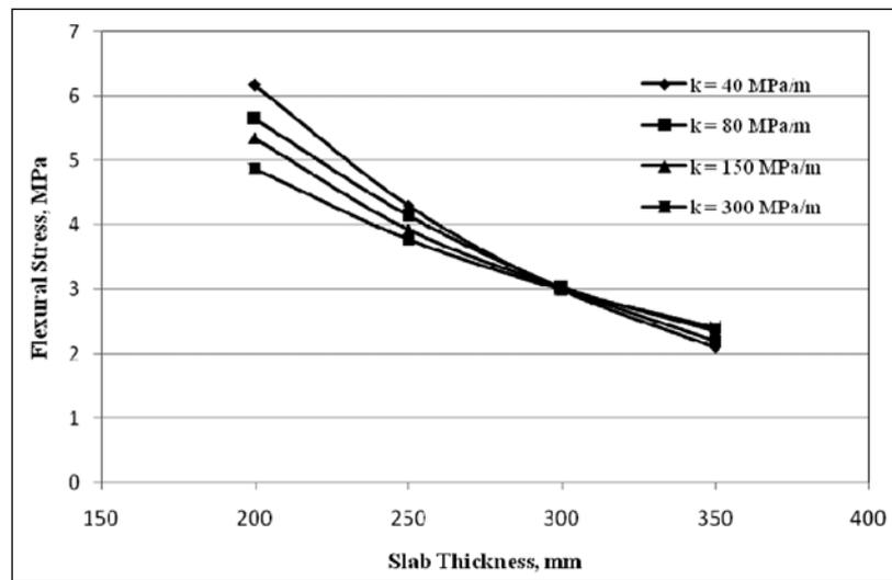
Fig. IV.20 Stress due to Single Axle Load of 200 kN,  $\Delta T = 17^\circ\text{C}$ , Without Concrete Shoulder
