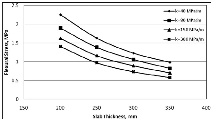
Fig. IV.53 Stress due to Tandem Axle Load of 200 kN,  $\Delta T = 0^\circ\text{C}$ , Without Concrete Shoulder
