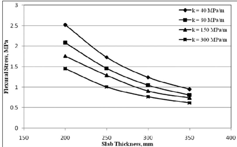
Fig. IV.28 Stress due to Single Axle Load of 120 kN,  $\Delta T = 0^\circ\text{C}$ , With tied Concrete Shoulder
