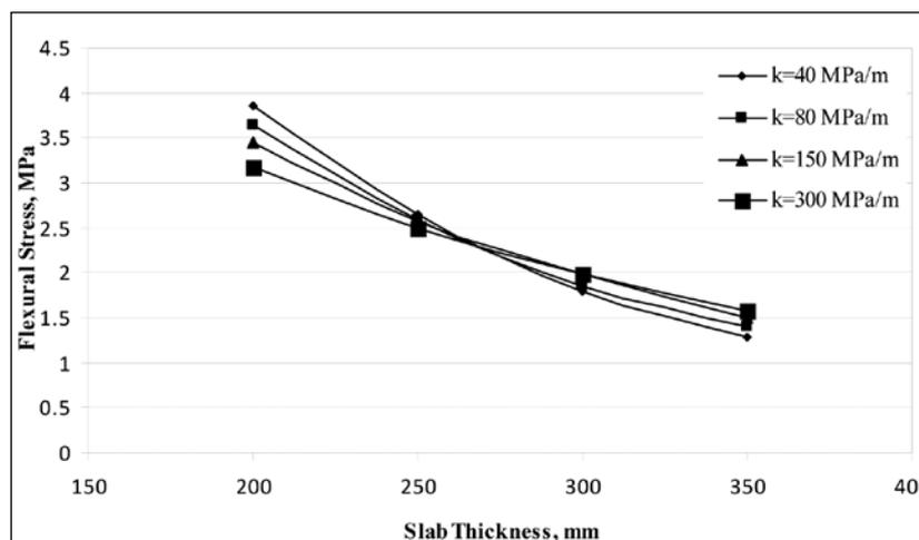
Fig. IV.12 Stress due to Single Axle Load of 120 kN,  $\Delta T = 13^\circ\text{C}$ , Without Concrete Shoulder
