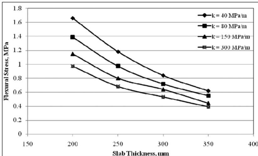
Fig. IV.27 Stress due to Single Axle Load of 80 kN, ΔT = 0°C, With Tied Concrete Shoulder
