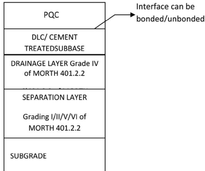
Fig. VII.1 Typical Cross-Section of Concrete Pavement
