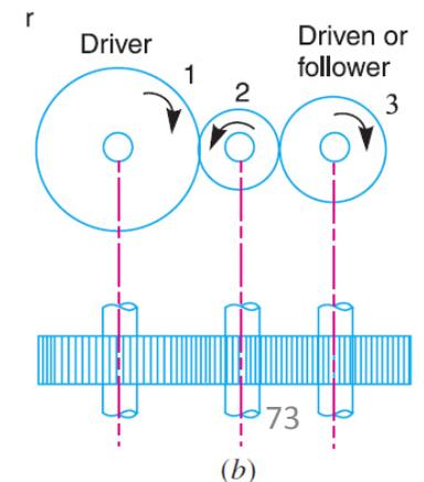
Similarly, it can be proved that the above equation holds good even if there are any number of intermediate gears. From above, we see that the speed ratio and the train value, in a simple train of gears, is independent of the size and number of intermediate gears. These intermediate gears are called *idle gears*, as they do not effect the speed ratio or train value of the system. The idle gears are used for the following two purposes :
