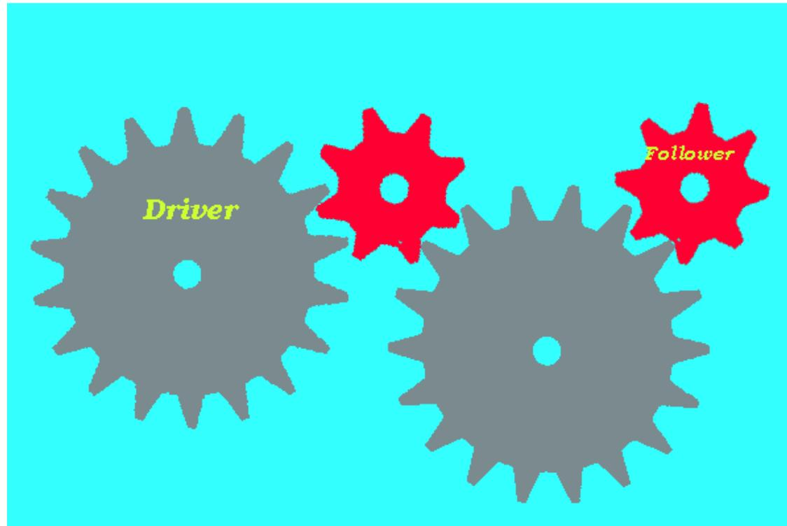
Since the speed ratio (or velocity ratio) of gear train is the ratio of the speed of the driver to the speed of the driven or follower and ratio of speeds of any pair of gears in mesh is the inverse of their number of teeth, therefore
