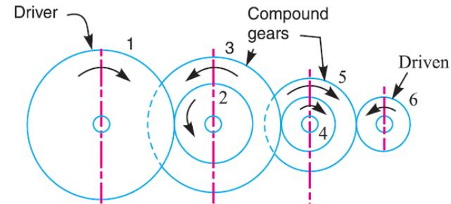
The speed ratio of compound gear train is obtained by multiplying the equations (i), (ii) and (iii),
