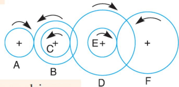
$$\frac{\text{Speed of the first driver}}{\text{Speed of the last driven}} = \frac{\text{Product of no. of teeth on drivens}}{\text{Product of no. of teeth on drivers}}$$
