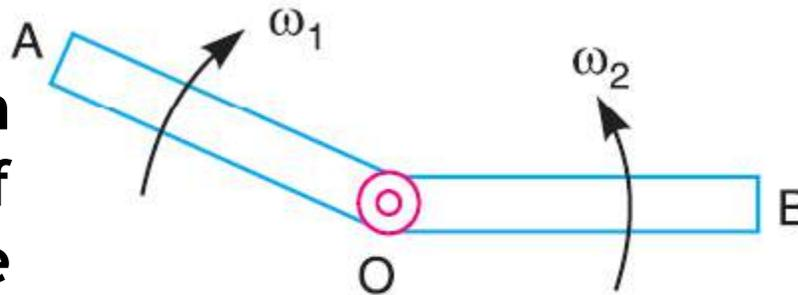
Links connected by pin joints.
