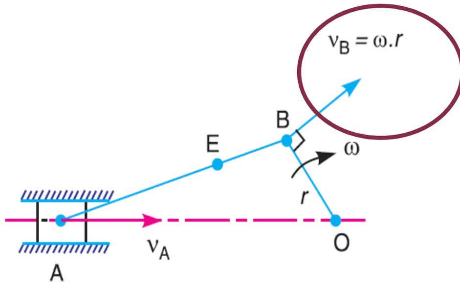
(a) Slider crank mechanism.
