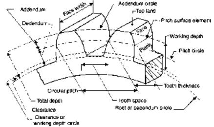
*Working depth:* It is the radial distance from the addendum circle to the clearance circle. It is equal to the sum of the addendum of the two meshing gears.
