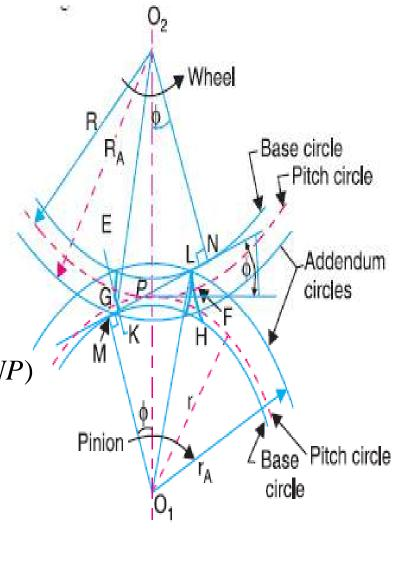
$$\therefore O_1 N = r \sqrt{1 + \frac{R}{r} \left(\frac{R}{r} + 2\right) \sin^2 \phi} = \frac{m t}{2} \sqrt{1 + \frac{T}{t} \left(\frac{T}{t} + 2\right) \sin^2 \phi}$$
