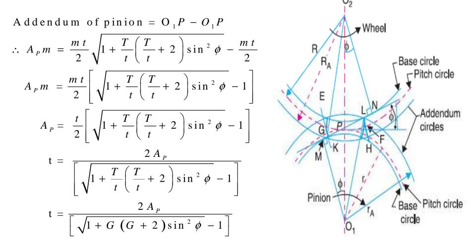
Two 20° involute spur gears mesh externally and give a velocity ratio of 3. Module is 3 mm and the addendum is equal to 1.1 module. If the pinion rotates at 120 rpm, determine (i) the minimum number of teeth on each wheel to avoid interference (ii) the number of pairs of teeth in contact. (ii) Contact ratio or number of pairs of teeth in
