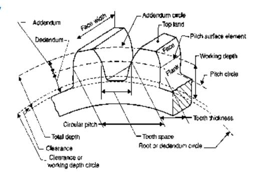
*Face of tooth:* It is the surface of the gear tooth above the pitch surface. *Flank of tooth:* It is the surface of the gear tooth below the pitch surface.
