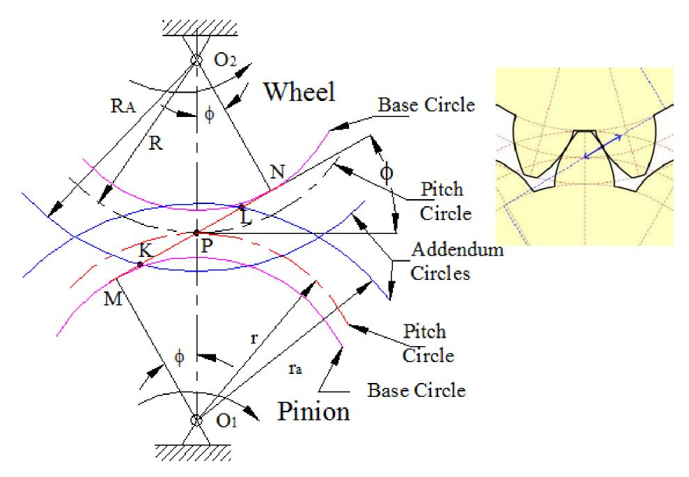
**Circular pitch:** It is the distance measured on the circumference of the pitch circle from a point of one tooth to the corresponding point on the next tooth. It is usually denoted by  $P_c$ , Mathematically,
