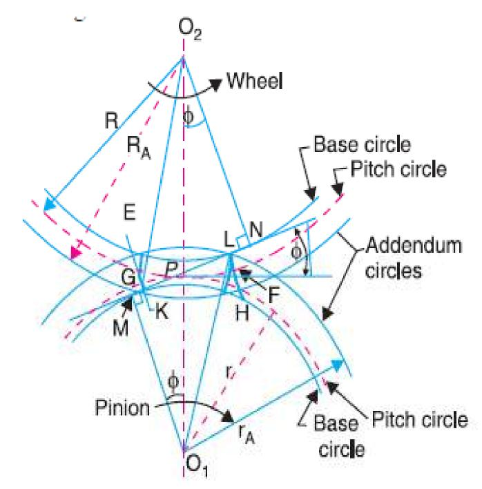
•MN is the common normal at the point of contact and the common tangent to the base circles.
