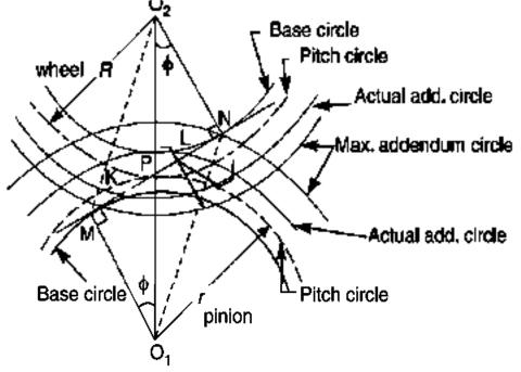
only be avoided, if the point of contact between the two teeth is always on the involute profiles of both the teeth. In other words, *interference may only be prevented, if the addendum circles of the two mating gears cut the common tangent to the base circles between the points of tangency.*
