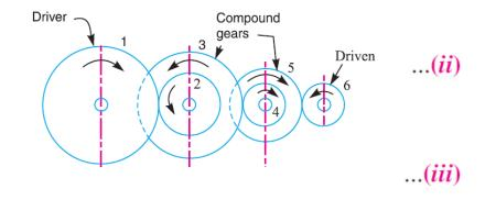
The speed ratio of compound gear train is obtained by multiplying the equations (i), (ii) and (iii),
