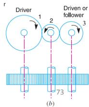
Similarly, it can be proved that the above equation holds good even if there are iny number of intermediate gears. From above, we see that the speed ratio and the rain value, in a simple train of gears, is inlependent of the size and number of internediate gears. These intermediate gears are called *idle gears*, as they do not effect the speed ratio or train value of the system. The dle gears are used for the following two purposes :
